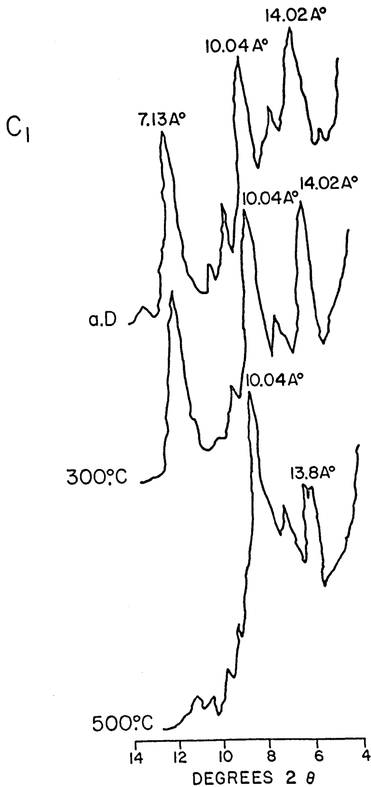
Figure 17. Diffractograms of Springerville gravelly clay, C 1 horizon (2-8"), coarse clay, K-saturated and heated to 300° and 500°C.
