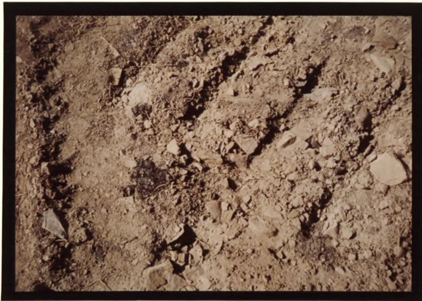
Figure 6. Close-up view of coal mining spoils material. -- This picture illustrates the type of soils material which is left after mining. One may note numerous bits of rock and coal mixed into the material which is left on the surface after mining.
