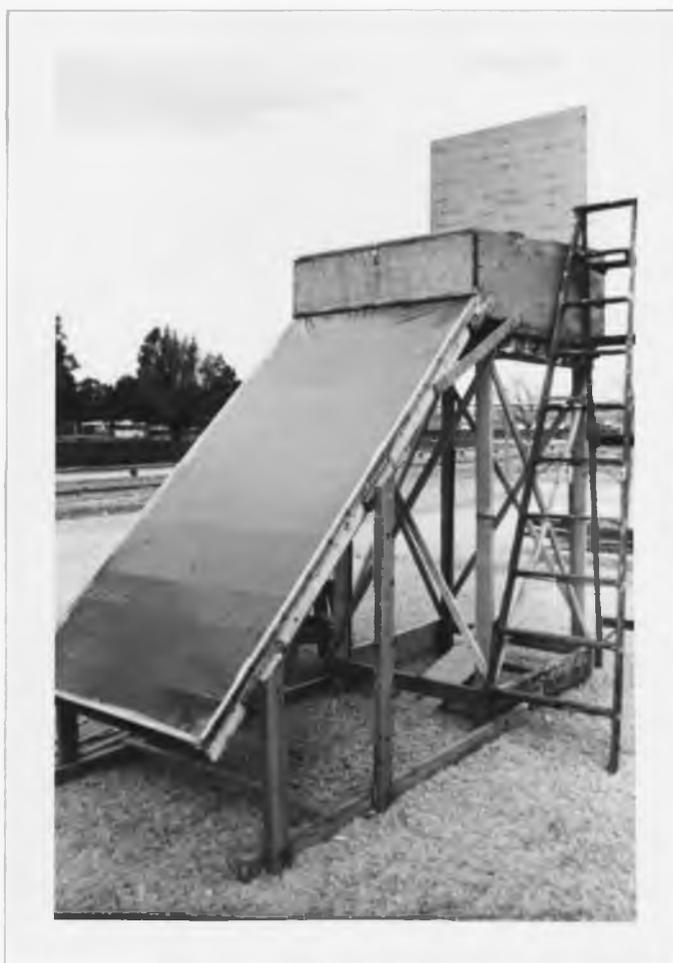
Figure 3. Proto dryer for tests at Campbell Avenue Farm.
