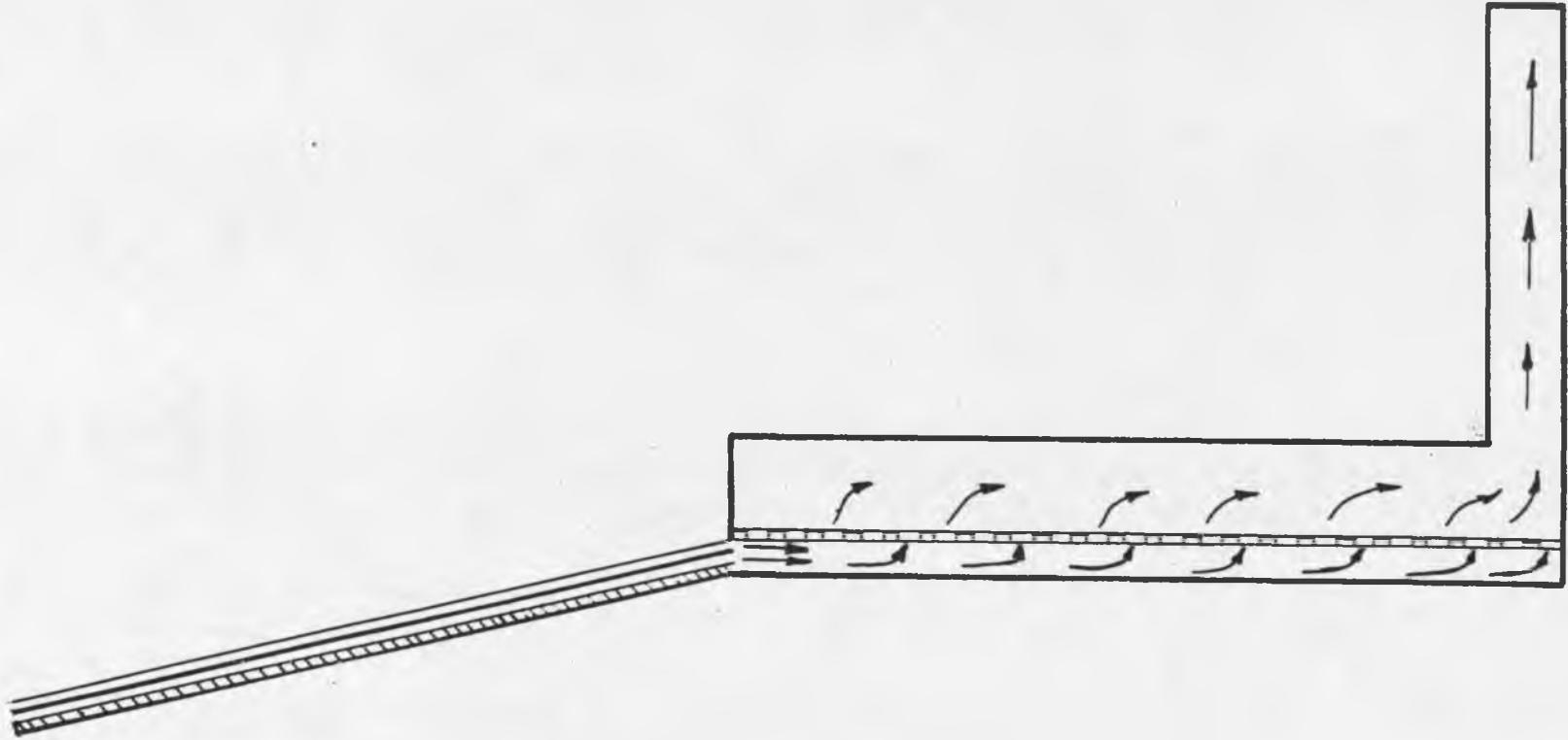
Figure 2. Cross section of solar grain drier.
