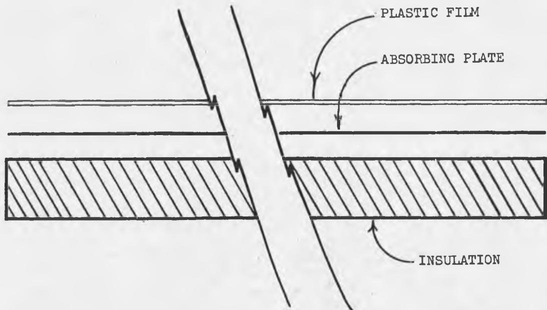
Figure 1. Cross section of solar collector.
