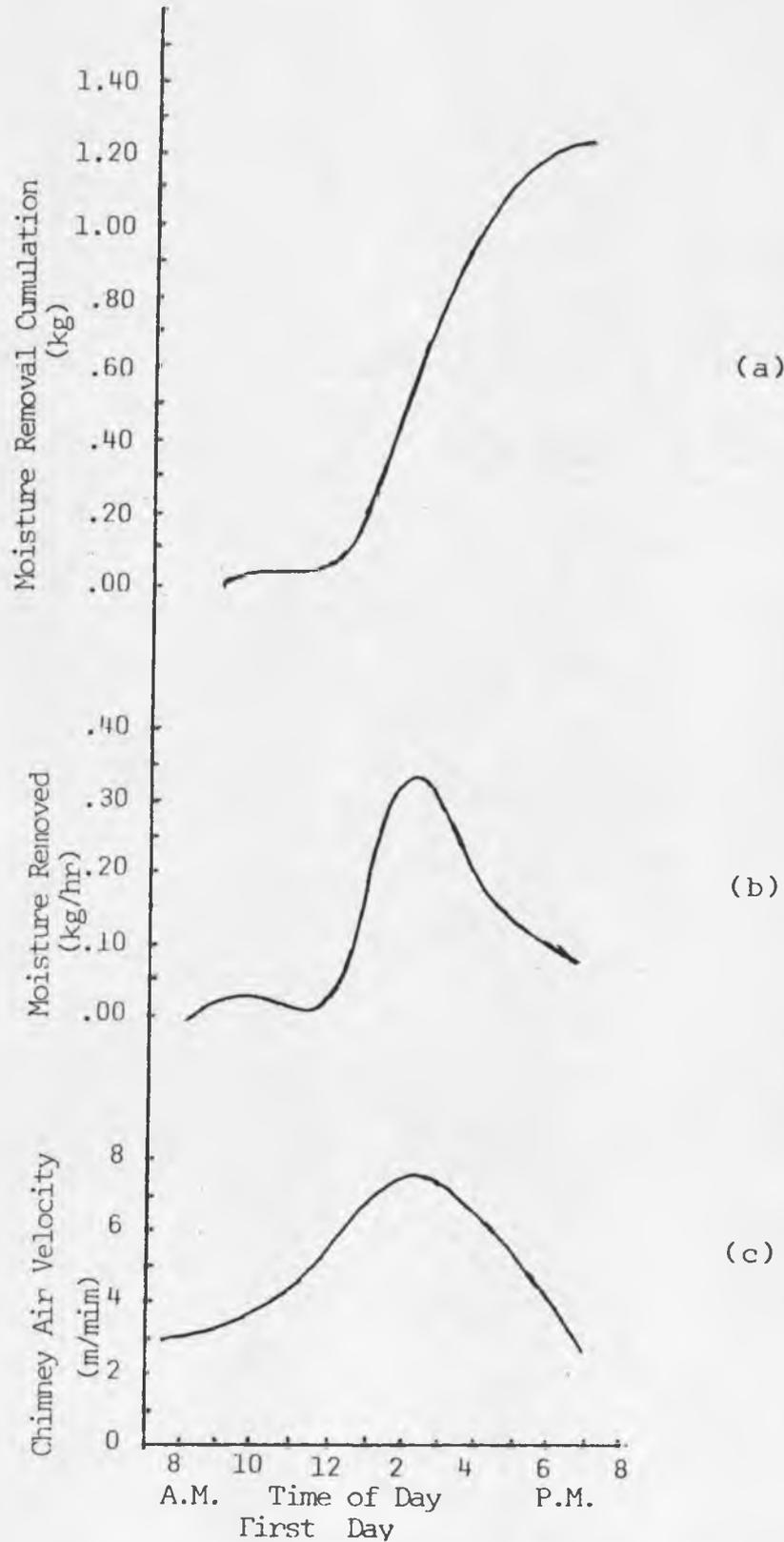
Figure 4. Moisture removal and chimney air velocity during first day of test.
