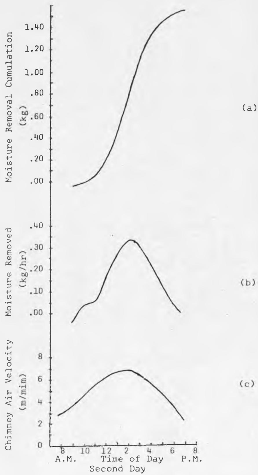
Figure 5. Moisture removal and chimney air velocity during second day of test.
