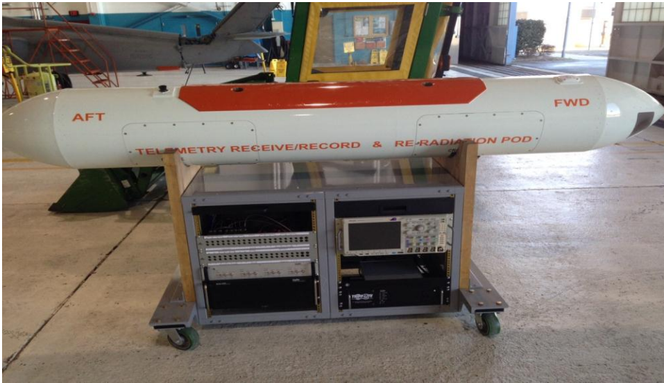
Figure 11.0 Telemetry Receive/Record Pod with Pod Cradle & Equipment Rack
