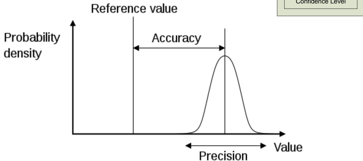
Precision, as demonstrated in the figure, represents the dispersion of values when repeated measurements are taken. The accuracy represents the proximity of the measurement values to the true value. Uncertainty includes both accuracy and precision as defined above and must be accompanied by a confidence interval to be of value.
