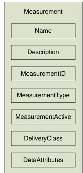
DataAttributes is a container within the Measurement element which has many more elements worth further discussion. Specification of units are done here as well as UnitConversions, which are specified as references to any number of DataOperation elements. As these are only references to other elements there are no issues to discuss at this point.
