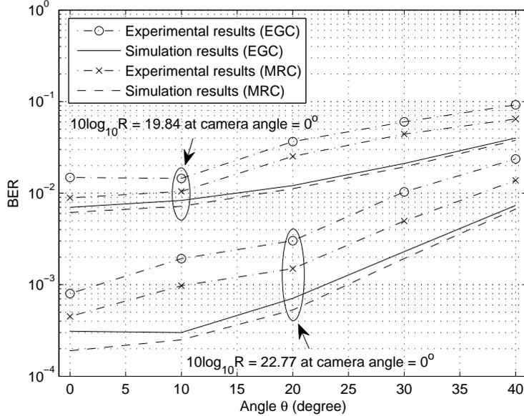
Fig. 6. BER performance at a distance  $d = 1$  m,  $f = 4.9$  mm for different camera angles  $\theta$ . BER performance is shown for two fixed values of  $10\log_{10}(R)$ .
