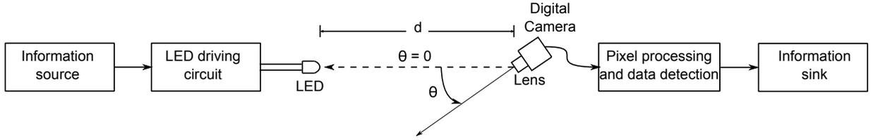
Fig. 1. An optical communication system using a digital camera as a receiver and an LED as a transmitter.
