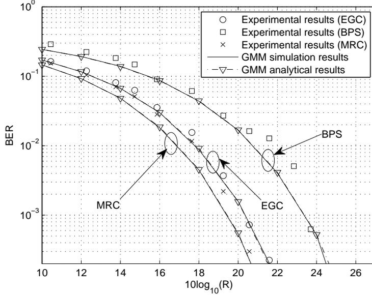
Fig. 4. BER performance at a distance  $d = 2$  m,  $\theta = 0^\circ$ , and  $f = 9.8$  mm. The LED's image is centered in a pixel and kept fixed.
