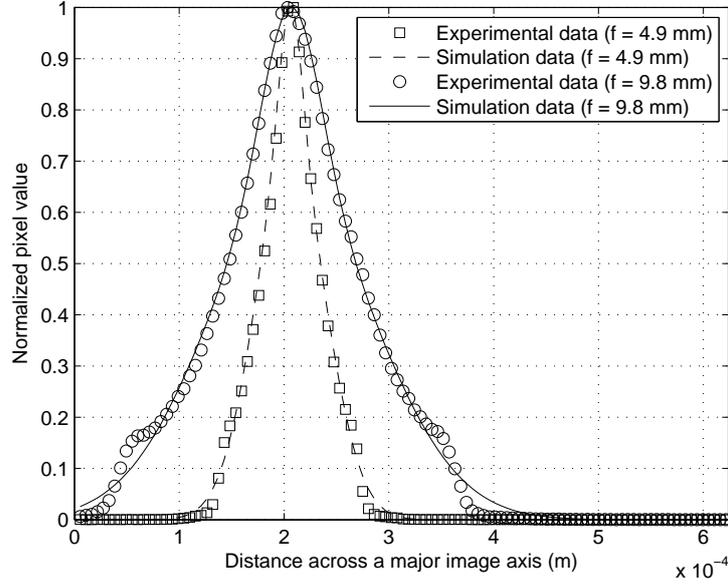
Fig. 2. GMM fit on the received LED image at  $d = 10$  cm and  $\theta = 0^\circ$  for  $f = 4.9$  mm and  $f = 9.8$  mm.
