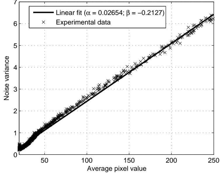
Fig. 3. Linear noise variance model for Promon 501 digital camera from AOS Technologies.
