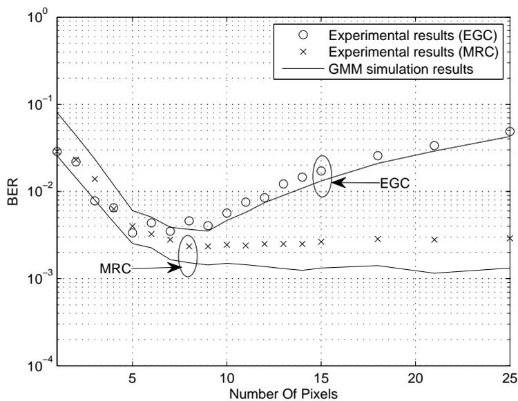
Fig. 5. BER performance at a distance  $d = 2$  m,  $\theta = 0^\circ$ , and  $f = 9.8$  mm using different numbers of pixels. The LED's image is centered in a pixel and kept fixed, and the transmitted power is fixed.
