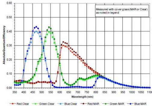
Figure 2: Spectral sensitivity of a typical CCD
