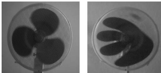
*Figure 1: Global shutter (clear) and rolling shutter (distorted)*
