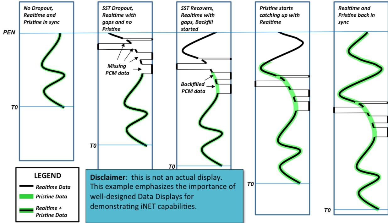
Figure 2. Example Stripchart Data Demonstrating PCM Backfill Capability
