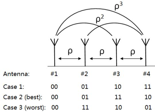
Fig. 3. Correlation among the transmit antennas and bit mappings for spatial modulation
