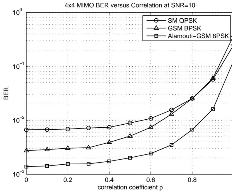
Fig. 8. BER vs. correlation coefficient  $\rho$  for SM, GSM and Alamouti-GSM for a  $4 \times 4$  MIMO system.  $N_a=2$  for GSM and Alamouti-GSM. The spectral efficiency is 4 bits/transmission
