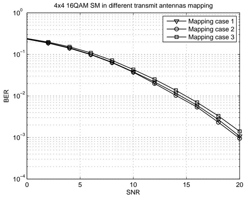
Fig. 9. SM for different bit-to-antenna mappings with  $4 \times 4$  MIMO and  $N_a = 2$ . The modulation is 16QAM and  $\rho=0.9$
