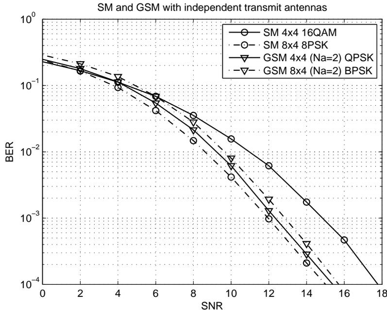
Fig. 5. SM and GSM with independent transmit antennas ( $\rho = 0$ ) with a spectral efficiency of 6 bits/transmission
