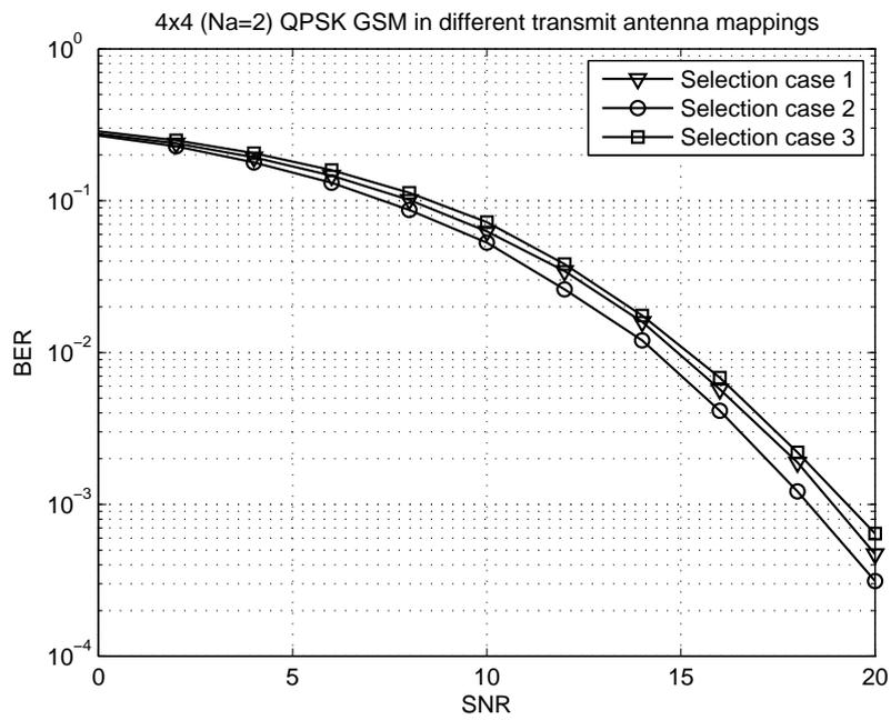
Fig. 10. GSM for different bit-to-antenna mappings with  $4 \times 4$  MIMO and  $N_a = 2$ . The modulation is QPSK and  $\rho=0.9$
