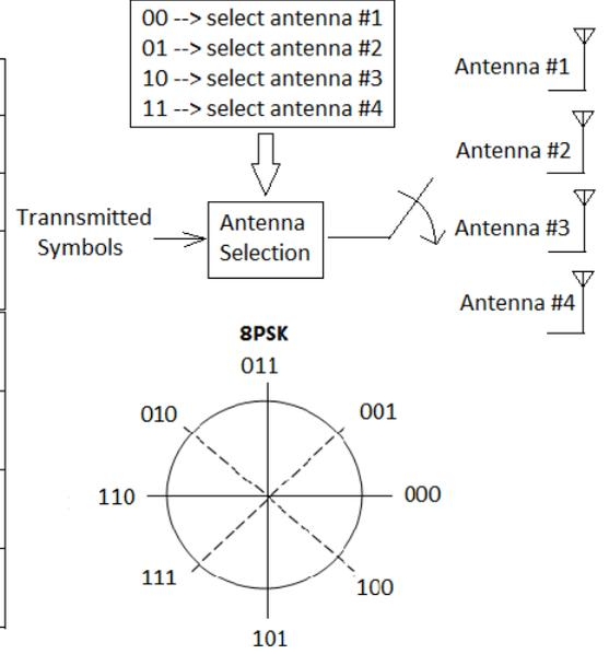
Fig. 1. Spatial modulation for a  $N_t=4$  system with 8PSK
