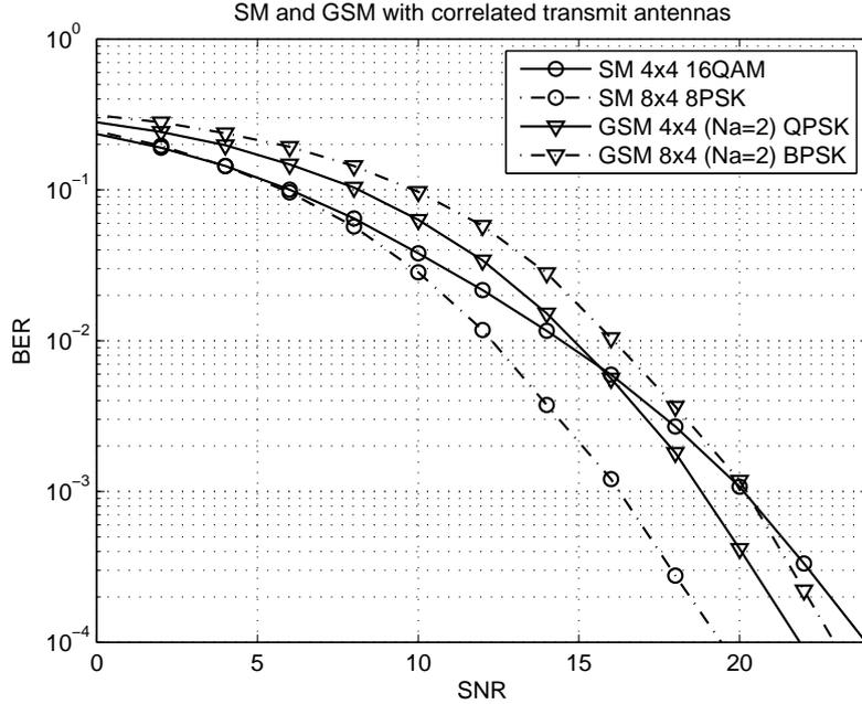
Fig. 6. SM and GSM with correlated transmit antennas ( $\rho=0.9$ ) for all cases, with a spectral efficiency of 6 bits/transmission
