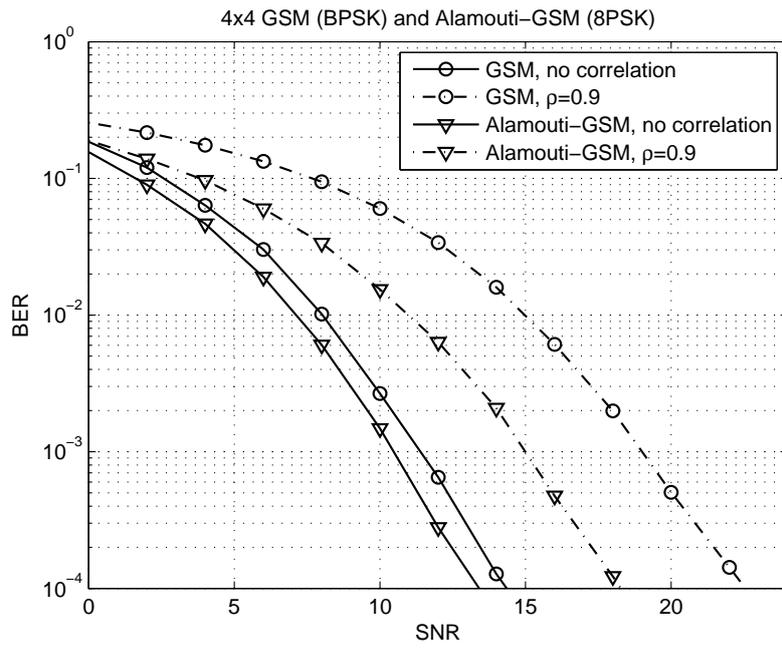
Fig. 7. GSM and Alamouti-GSM for a  $4 \times 4$  MIMO system with  $N_a=2$ . The spectral efficiency is 4 bits/transmission and  $\rho=0.9$
