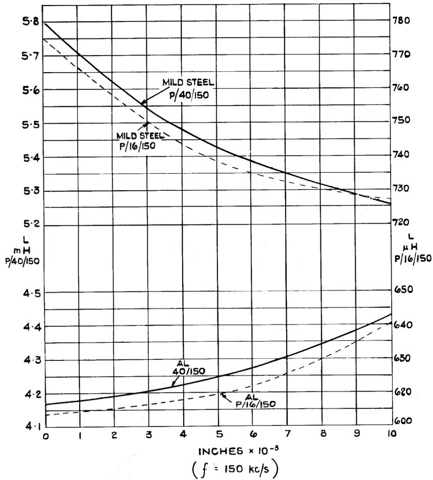
**Fig 4. Variation of Transducer Inductance with Armature Spacing Frequency 150 Kc/s**
