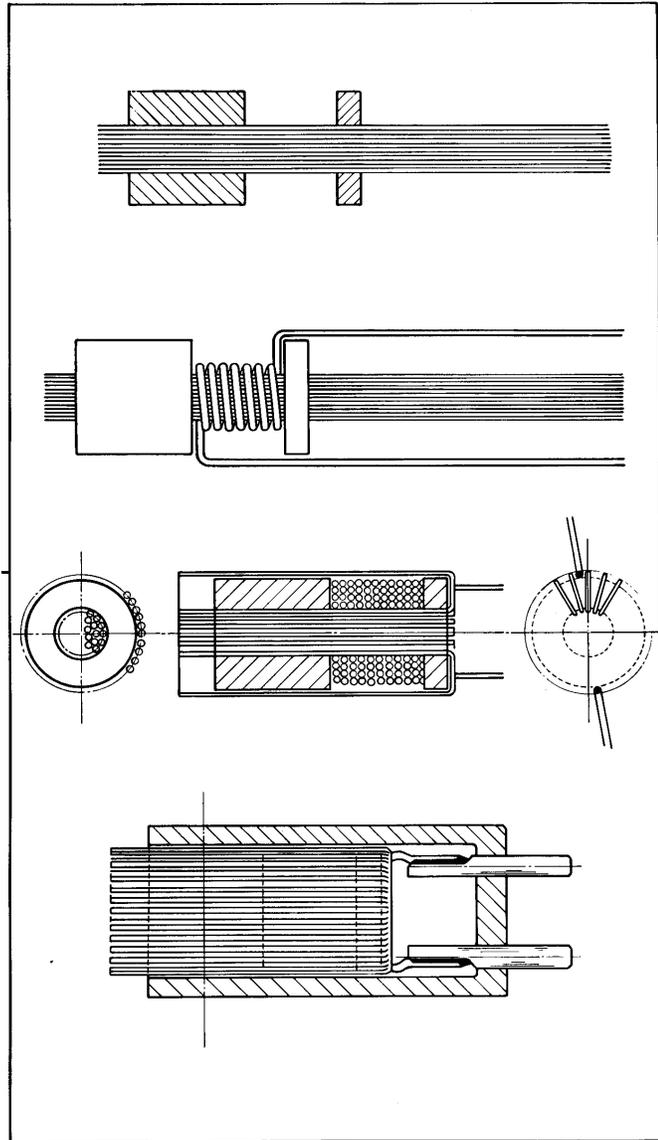
**Fig 1. Construction Stages of a Subminiature Inductive Transducer**
