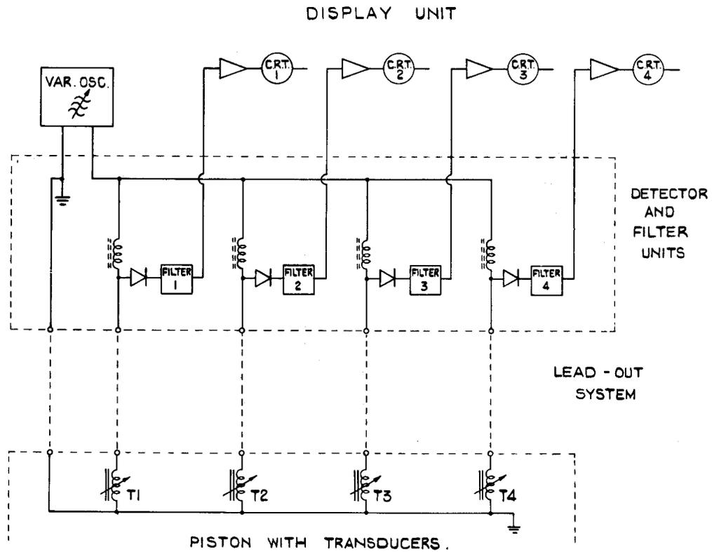
**Fig 5. Block Diagram of Instrumentation for Measurement of Piston Movement in an I.C. Engine**
