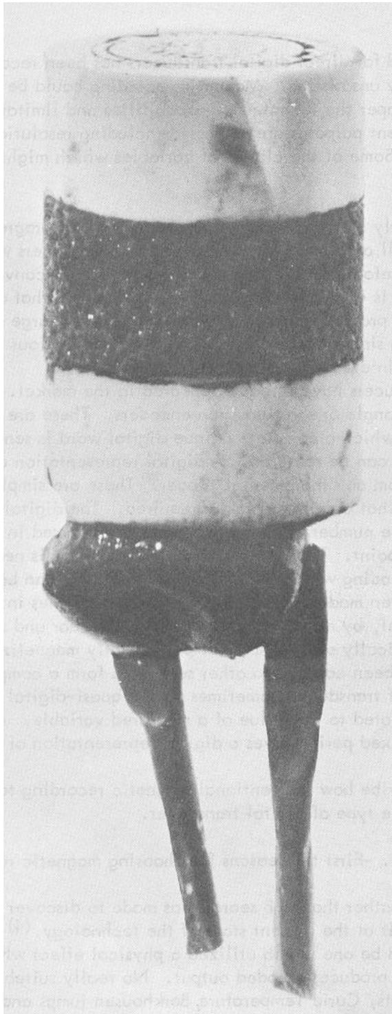
**Fig 9. High-Temperature Transducer P/40/600**
