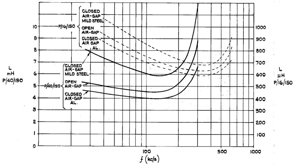
**Fig 3. Variation in Transducer Inductance with Carrier Frequency, Open Air-Gap, Steel and Aluminim as Armature Material**
