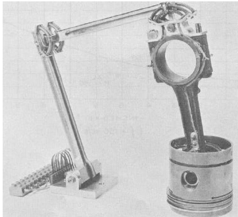
**Fig 6. Piston Fitted with 4 Inductive Transducers and Lead-out System**
