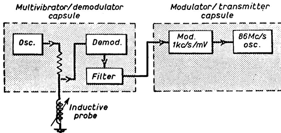
**Fig 8. F.M. Telemetry System with Inductive Transducer for the Measurement of Piston Movement in an I.C. Engine**
