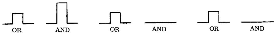
OUTPUTS OF THE OR AND AND LOGIC OF (a), (b), and (c) ABOVE
