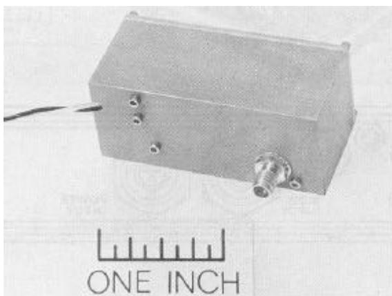
**Fig. 4-Crystal Oscillator-Multiplier-Mixer Module**
