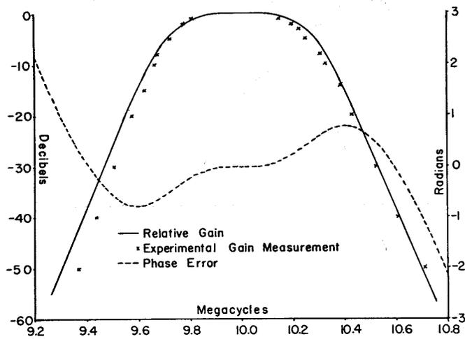
**Figure 3: Tuned Amplifier Characteristics**
