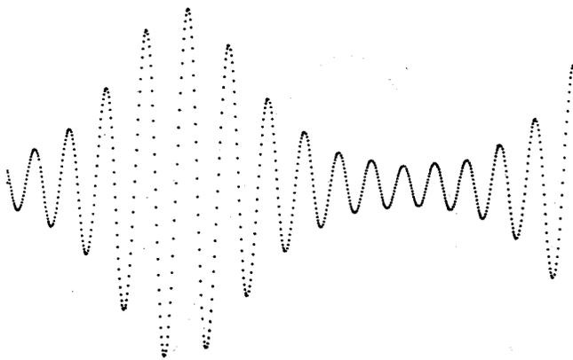
**Figure 2: Modulated 1 M. C. Carrier**
