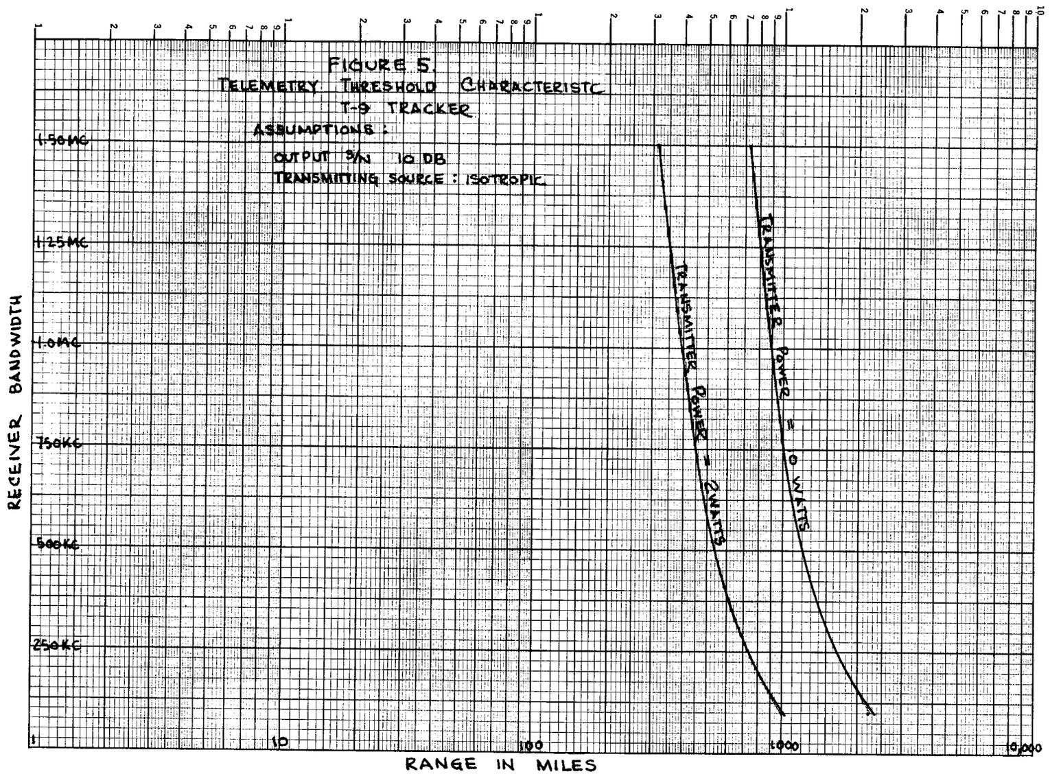
Figure 5. -Telemetry Threshold Characteristic T-9 Tracker
