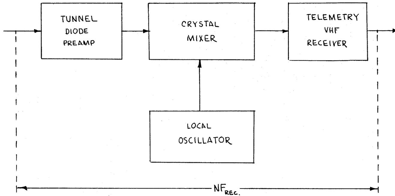
Figure 4. -RF System Block Diagram
