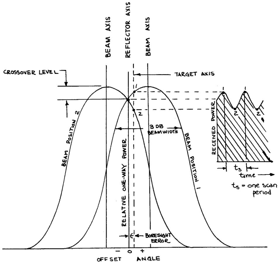
Figure 1. -A Typical Conical Scan Pattern
