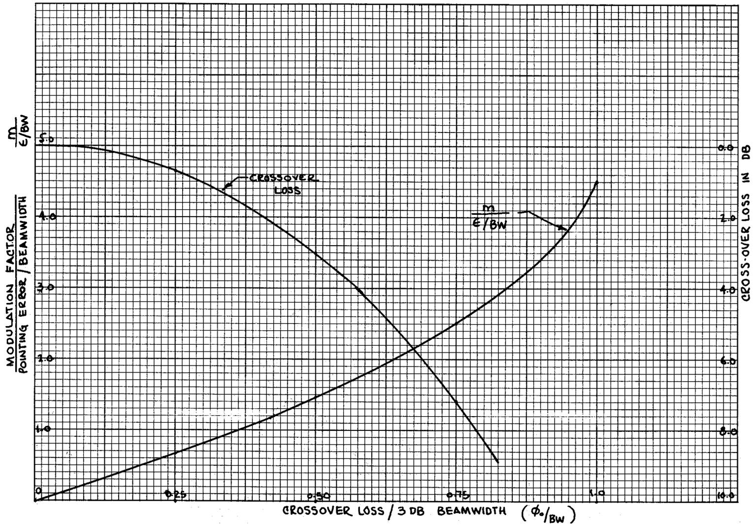
Figure 3. -Modulation Factor and Crossover Loss Versus Crossover Angle
