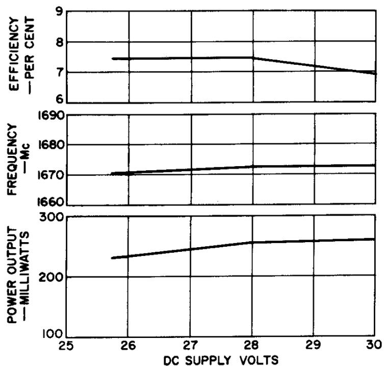
**Fig 7 - Power output, frequency, and efficiency of the TOM as a function of the dc supply voltage with a voltage regulator.**
