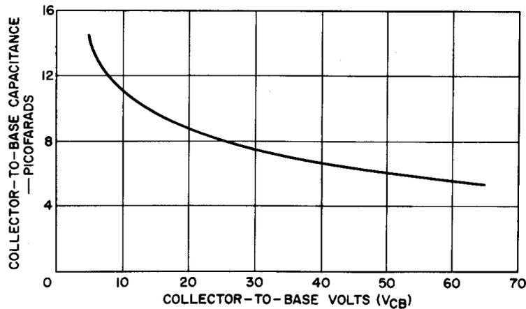
**Fig.2 -Collector-to-base junction capacitance of the RG4-210553 overlay transistor as a function of the voltage applied across the junction.**
