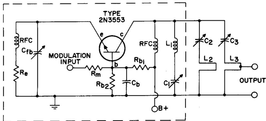
**Fig. 3 - Schematic of the S-131 L-band TOM power source.**
