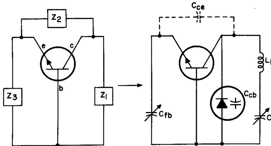
**Fig. 4 - AC equivalent circuits of the oscillator section of the TOM.**
