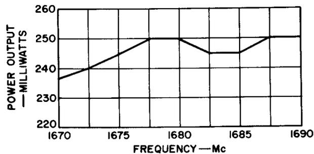
**Fig.10 -Power output as a function of frequency using mechanical single-screw tuning.**
