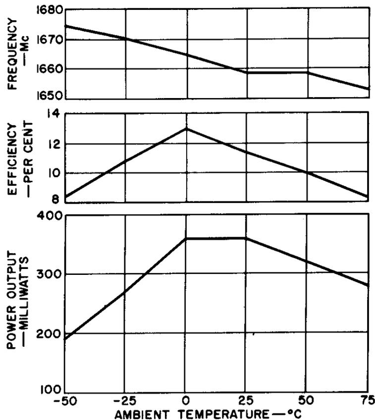
**Fig.8 -Power output, frequency, and efficiency of the TOM as a function of ambient temperature for a unit operated without temperature compensation and from an unregulated dc power supply.**
