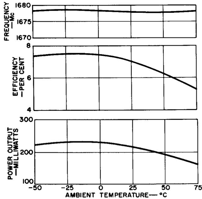
**Fig. 9 -Power output, frequency, and efficiency of the TOM as a function of ambient temperature for a temperature-compensated unit operated with a voltage regulator.**
