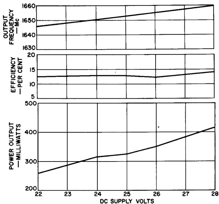
**Fig.6- Power output, frequency, an efficiency of the TOM as a function of the supply voltage without regulation.**
