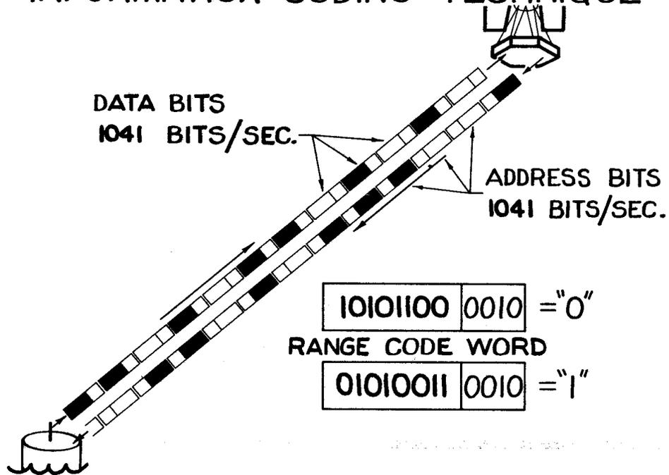
Fig. 9-Ranging Code and Information Modulation
