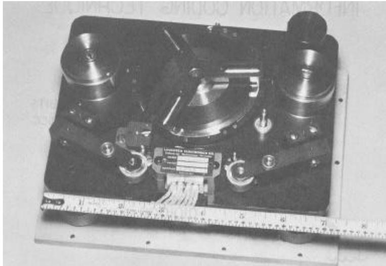
**Fig. 7-Digital Tape Recorder for Transverse PCM Recording**
