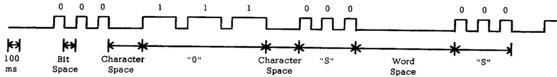
**Fig. 1 - PMCM (Pulse -Morse Code Modulation) Wavetrain**
