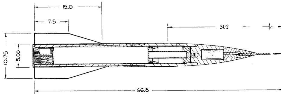
**Fig. 4. TMA payload and telemetry unit.**
