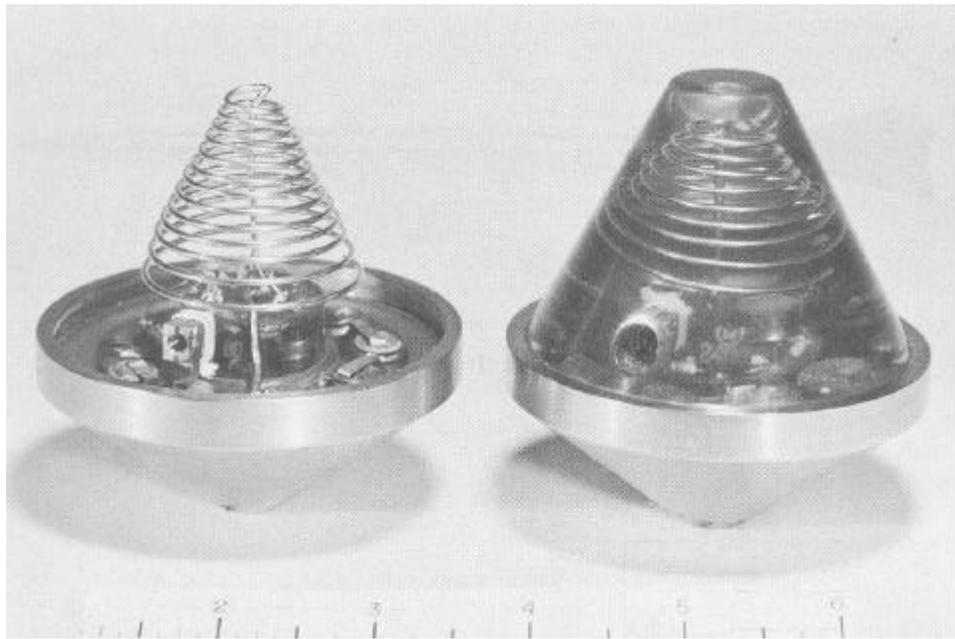
**Fig. 1. Model re-entry vehicle before and after potting.**
