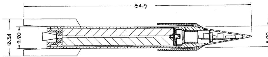
**Fig. 5. Rocket vehicle with magnetometer payload and telemetry.**
