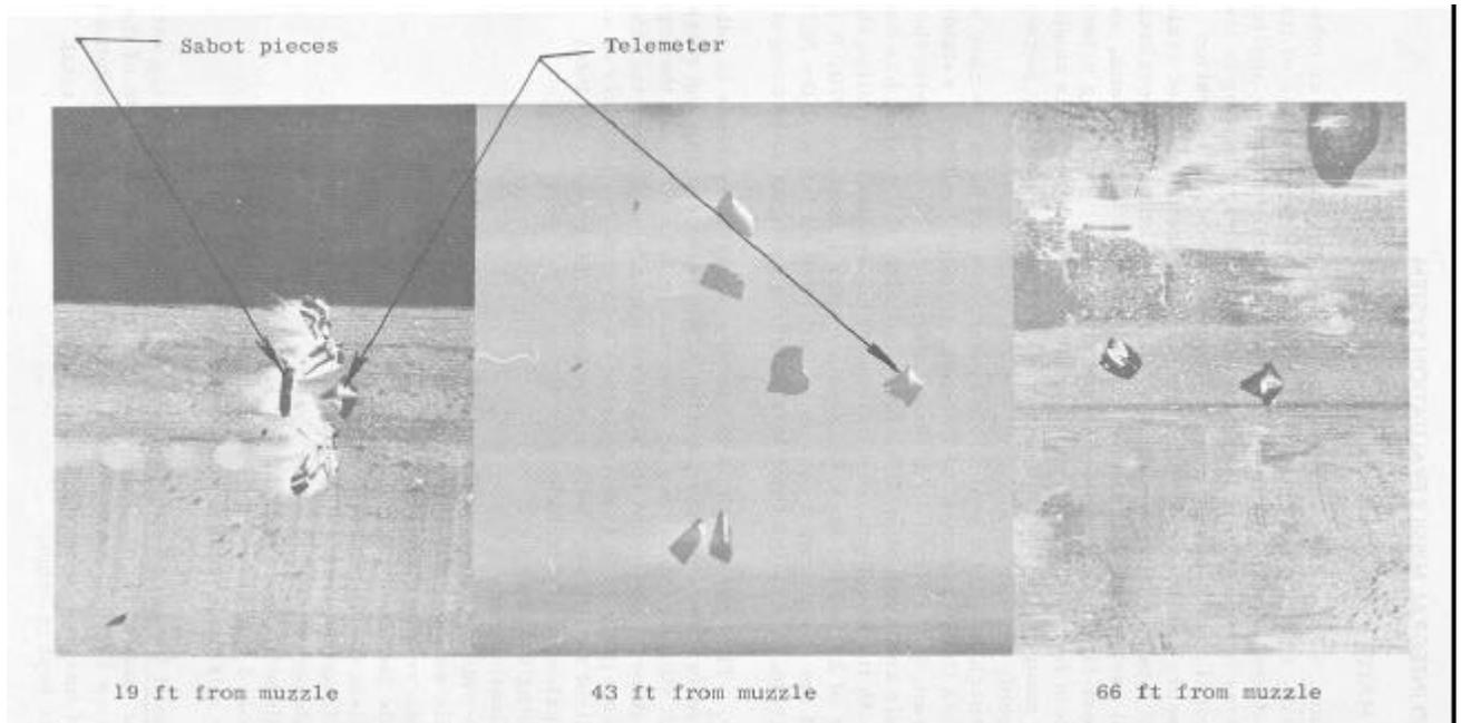
**Fig. 6. Missile-sabot separation (smear camera record), launch of temperature telemeter by BRL.**
