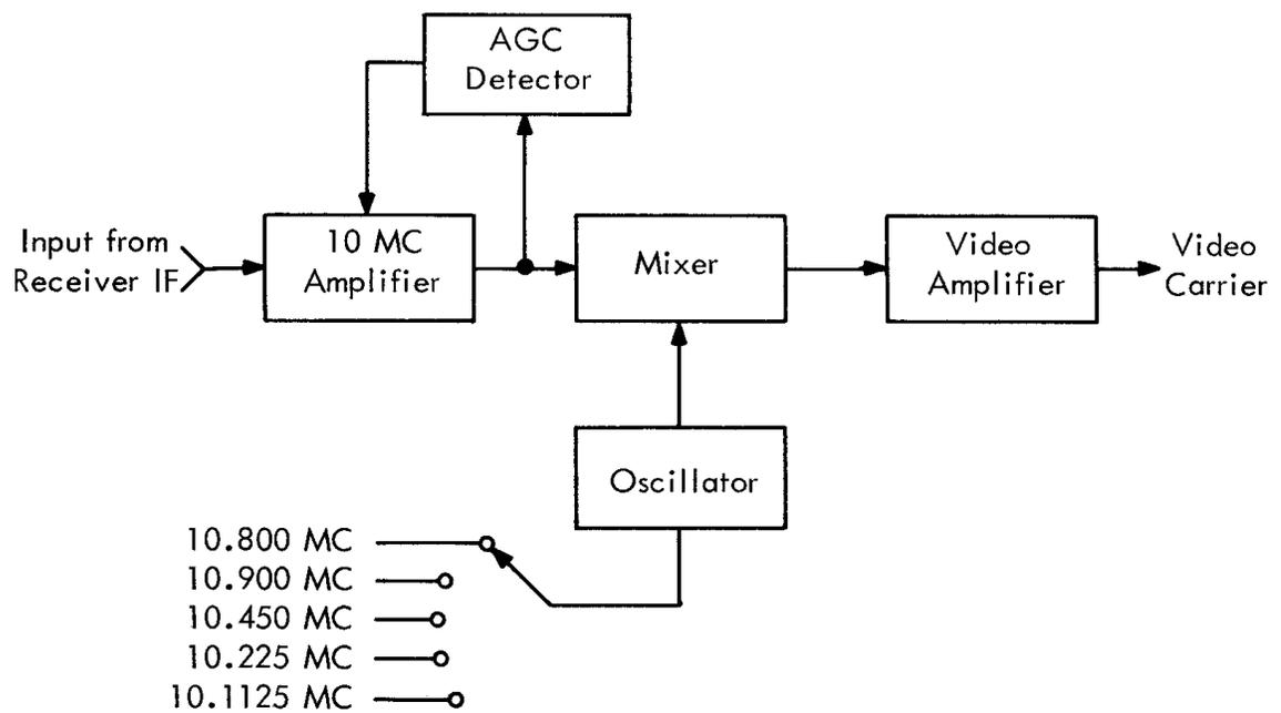
**Figure 2. Pre-D Record Module, Block Diagram**
