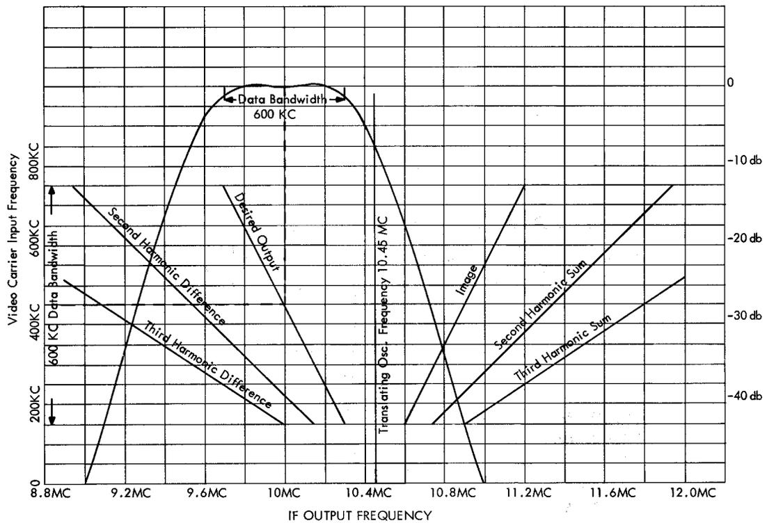
**Figure 4. Graphical Representation of Output Signal Components of Up-Translator Using 450 kc Video Carrier with Response 1 of 750 kc BW IF Amplifier Superimposed**
