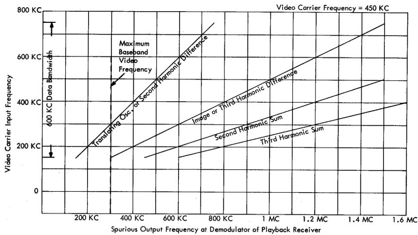
**Figure 5. Spurious Output Frequencies at the Demodulator of the Playback Receiver vs Instantaneous Video Carrier Frequency**
