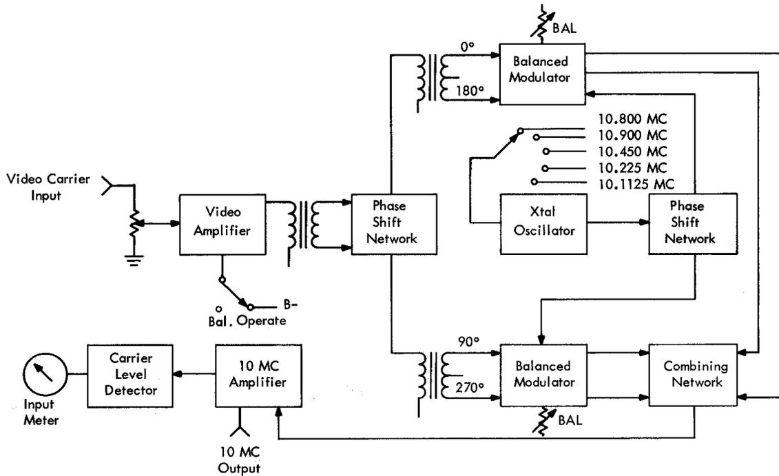
**Figure 3. Pre-D Playback Module, Block Diagram**
