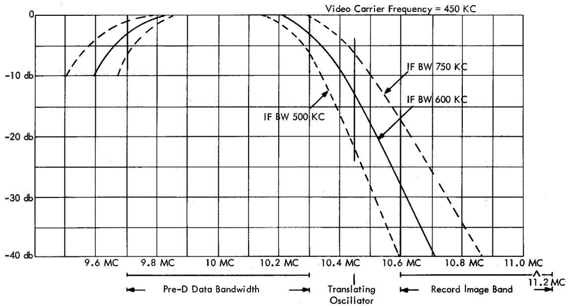
**Figure 7. Pre-D Record Image Band Rejection for Typical Receiver IF Bandwidths**
