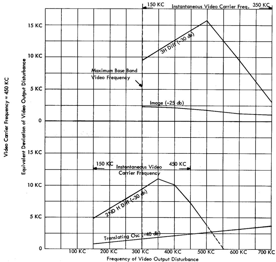
**Figure 6. Effect of Spurious Up-Translator Outputs at the Demodulator of the Playback Receiver**
