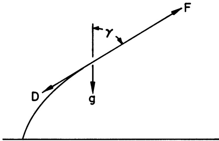
Figure 3. Forces Acting on Rocket
