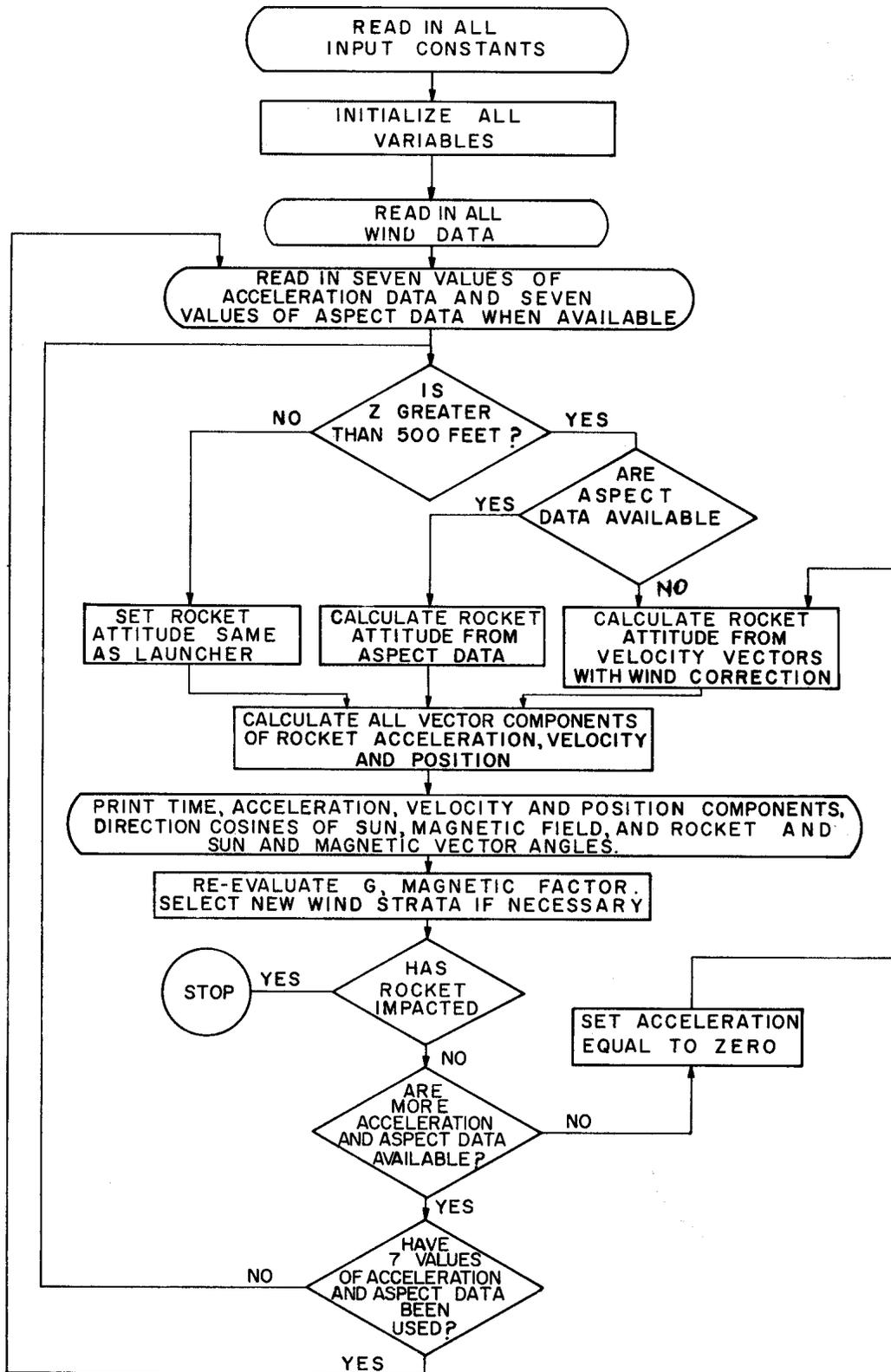
Figure 5. Simplified Flow Chart for Trajectory Program
