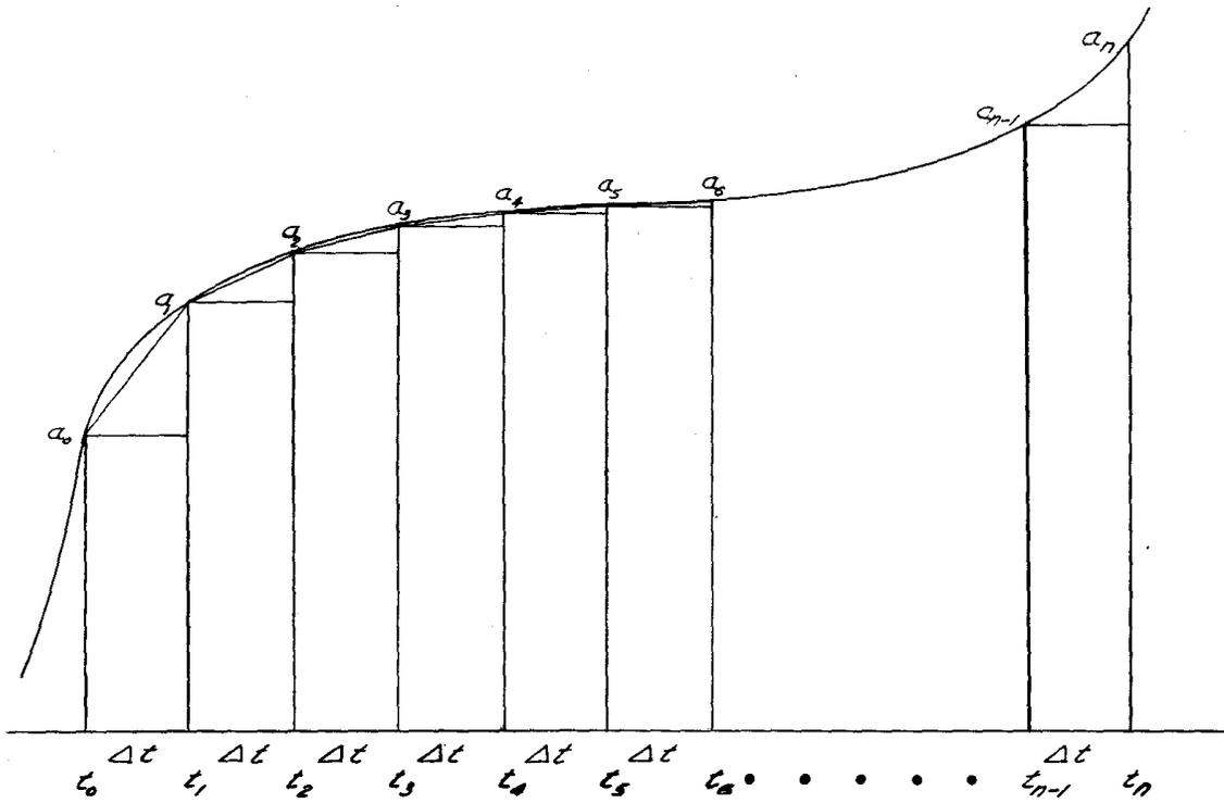
**Figure 1. Trapezoidal and Simpson's Rule Method for Numerical Integration**
