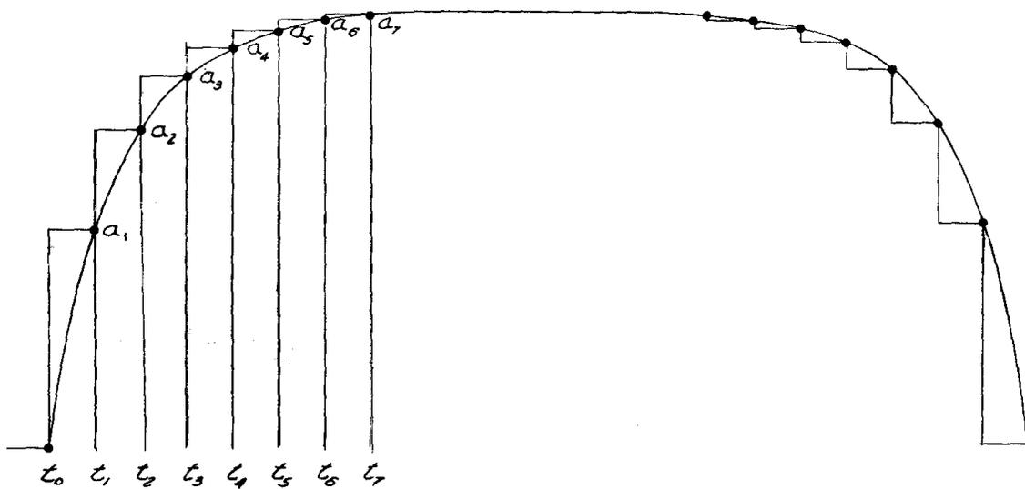
**Figure 2. Computer Method for Numerical Integration**
