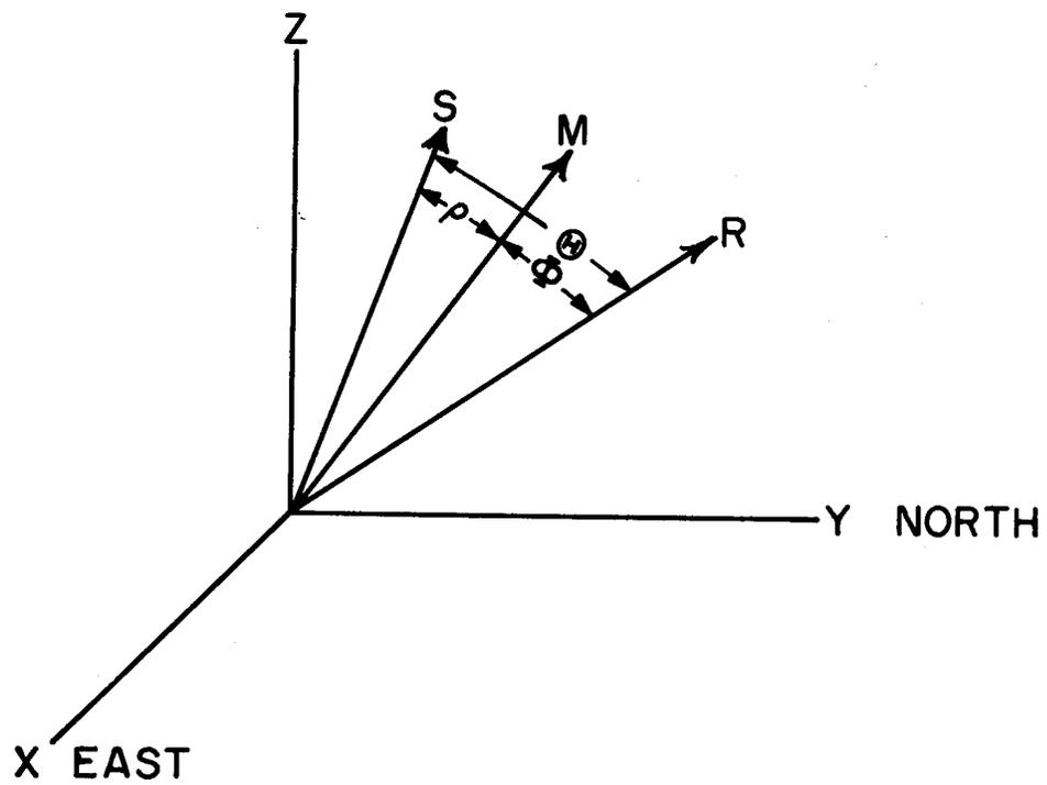
Figure 7. Sun, Magnetic Field, and Rocket Vector Diagram
