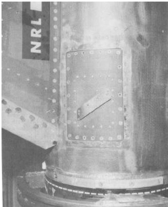
Figure 10. Solar Aspect Sensor Installed
