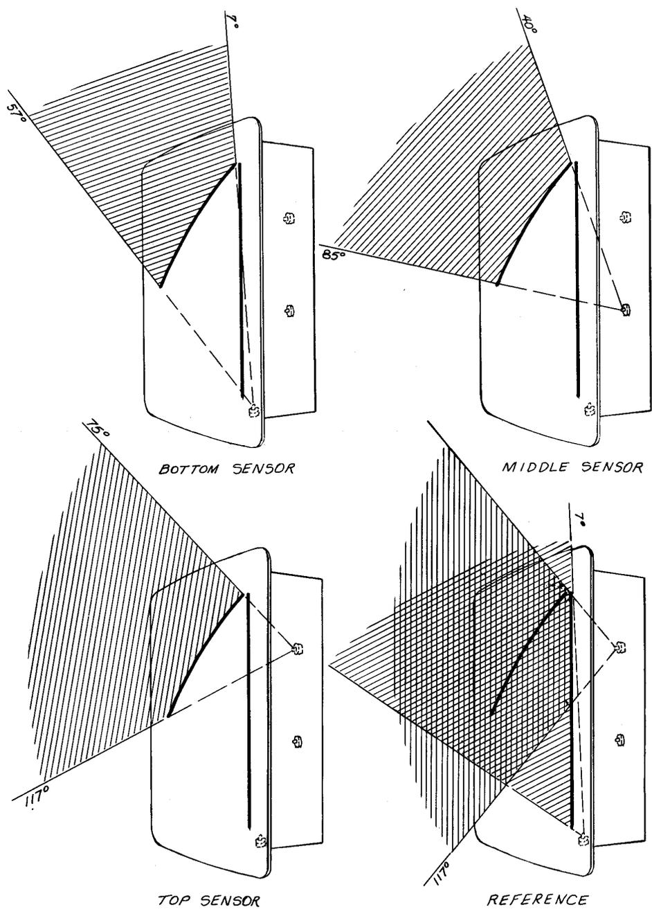
**Figure 8. Functional Sketches of Solar Aspect Sensor**
