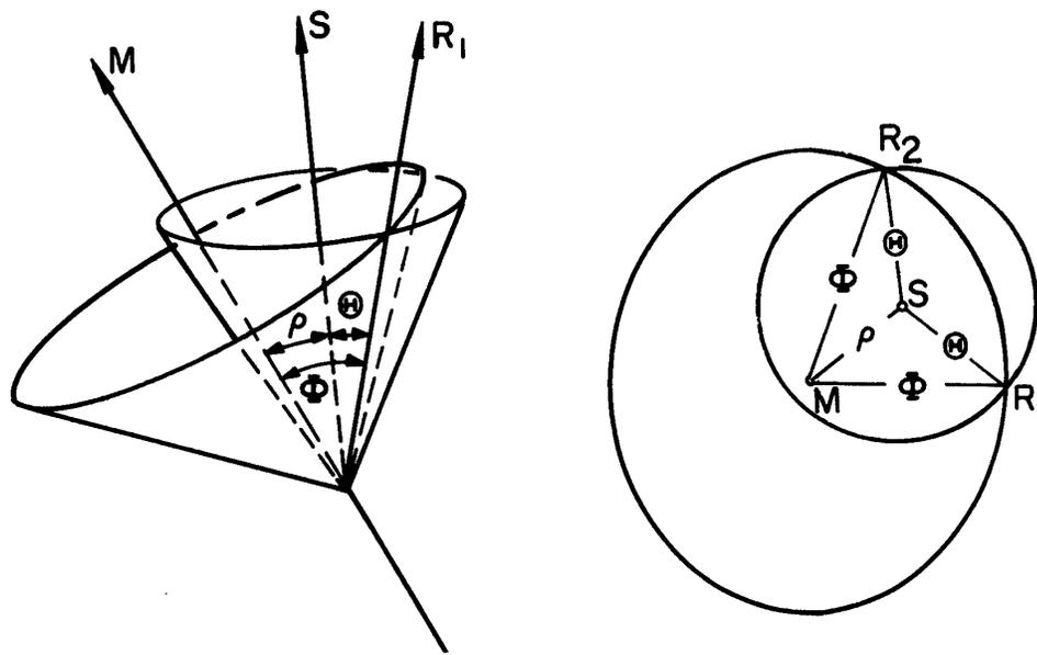
Figure 6. Intersecting Cone Representation of Rocket Vector
