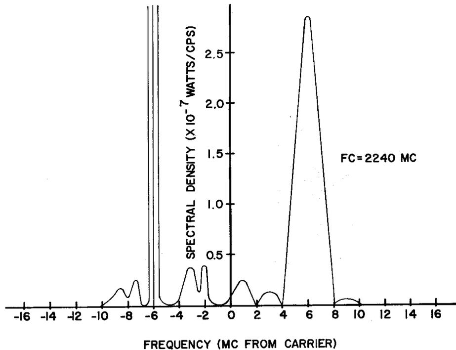
Figure A3. FM Spectrum of 500 ns. Non-Recurrent Pulse
