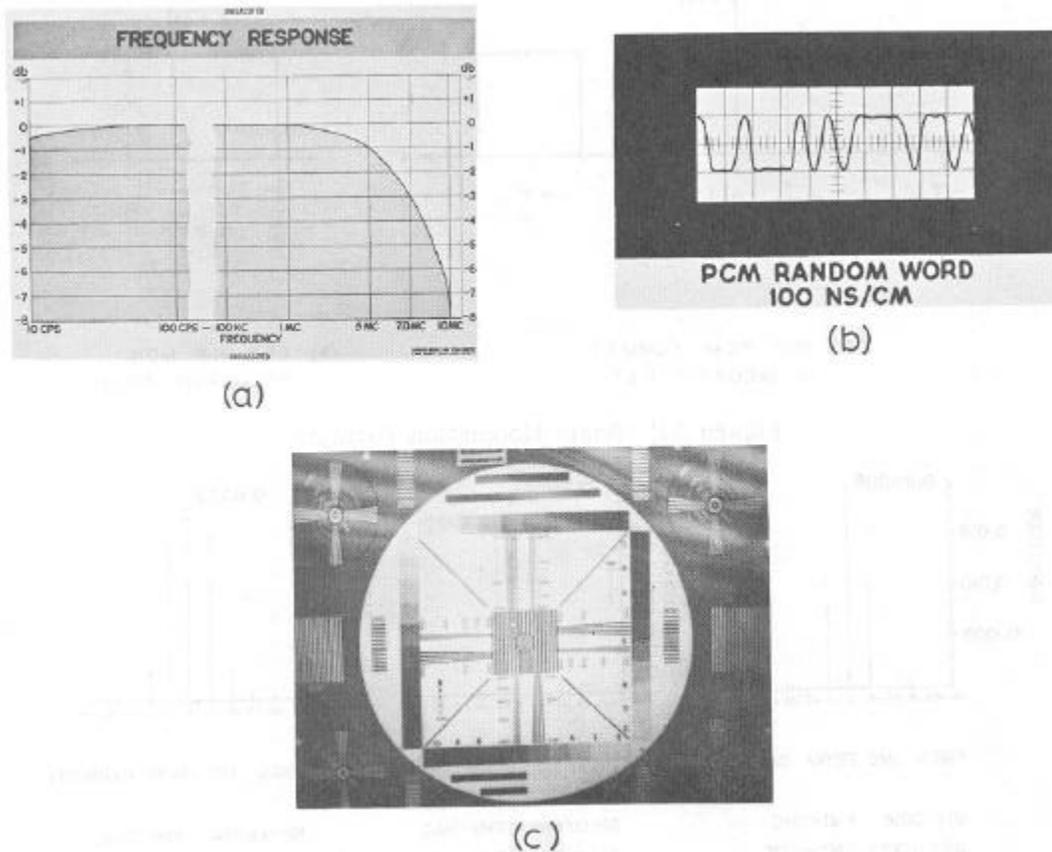
**Figure 2. Transmitter Performance (a) Frequency Response, (b) Megabit Digital Signal, (c) 525 Line Television Signal**
