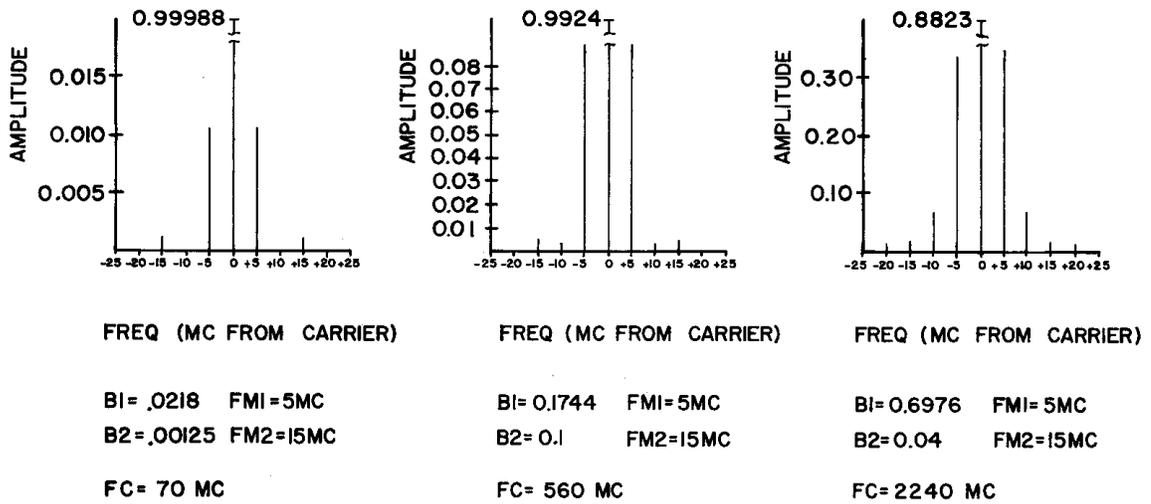
Figure A2. Two-Tone FM Spectra at Various Stages of the Transmitter
