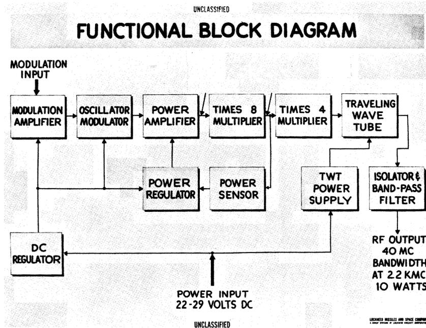
**Figure 1. Transmitter Block Diagram**
