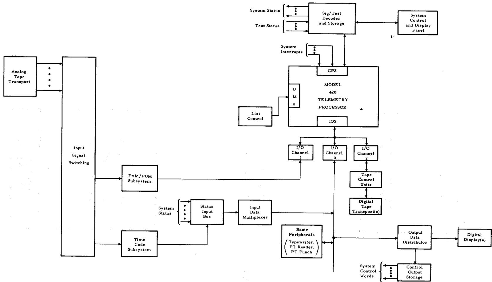
Figure 15. Model 8420 Configuration for Application Number Two (PAM/PDM Conversion)
