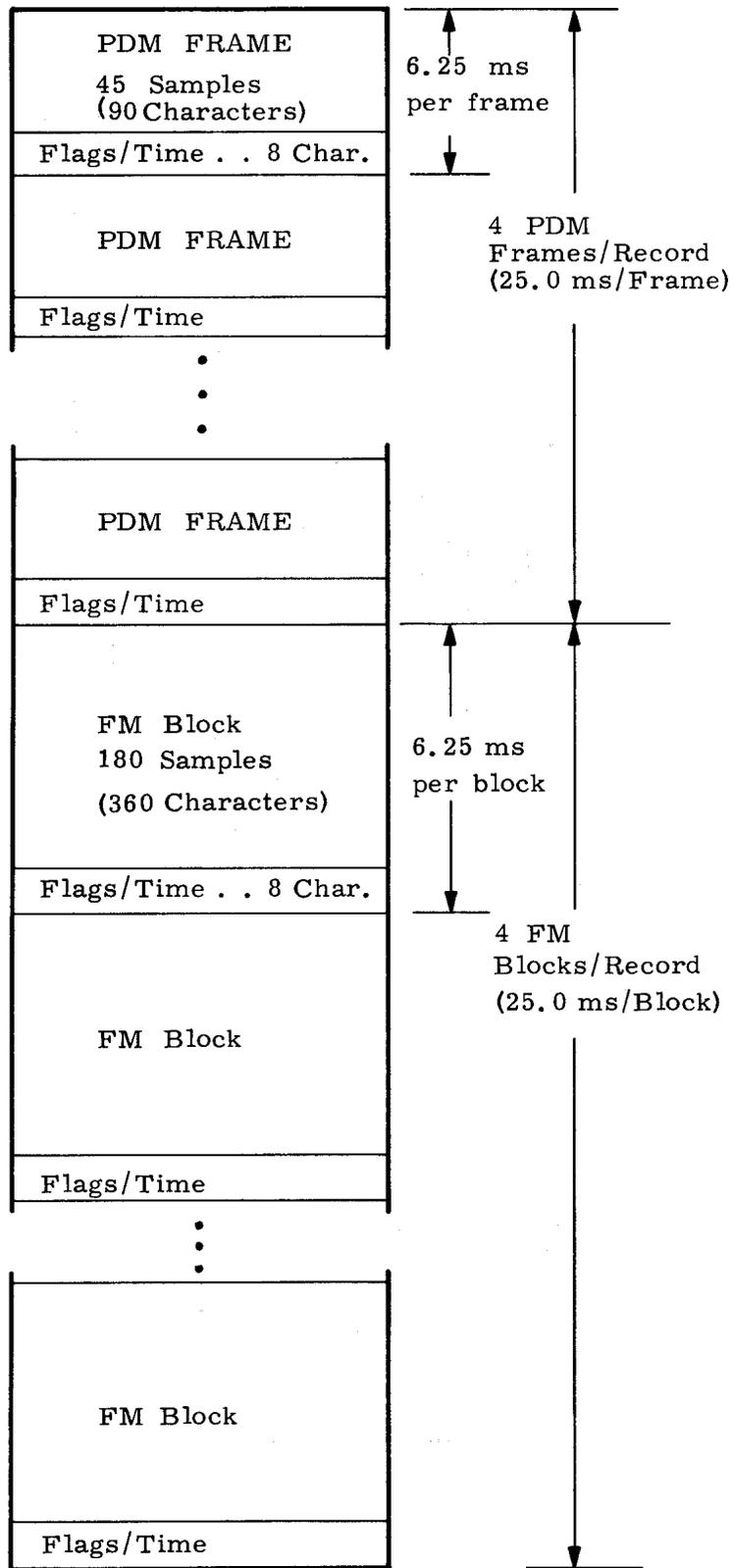
**Figure 20. Example 4. Output Tape Format, PDM/FM Merge Mode**
