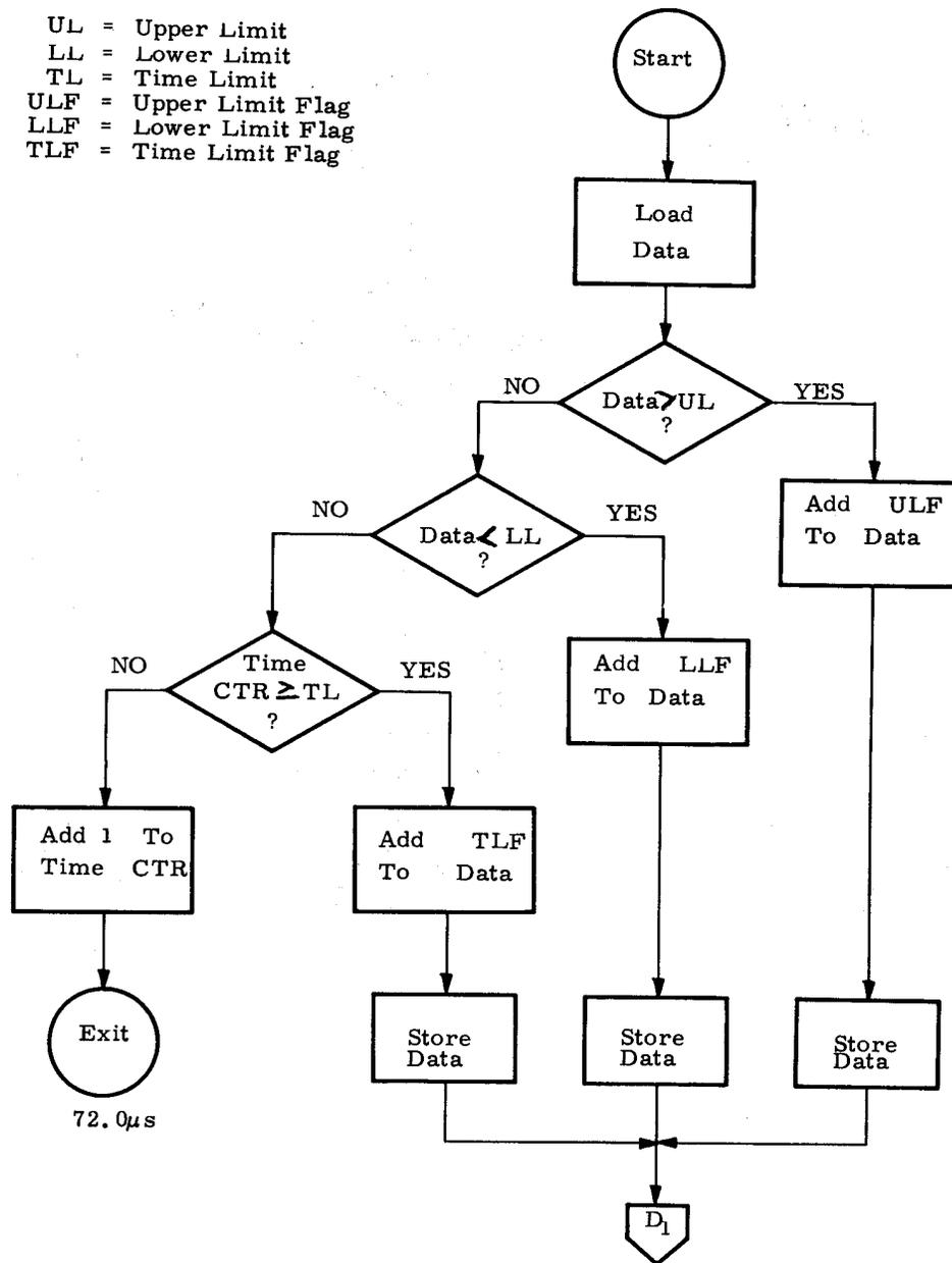
Figure 11. Data Compression (Resettable Limits) (1 of 2)
