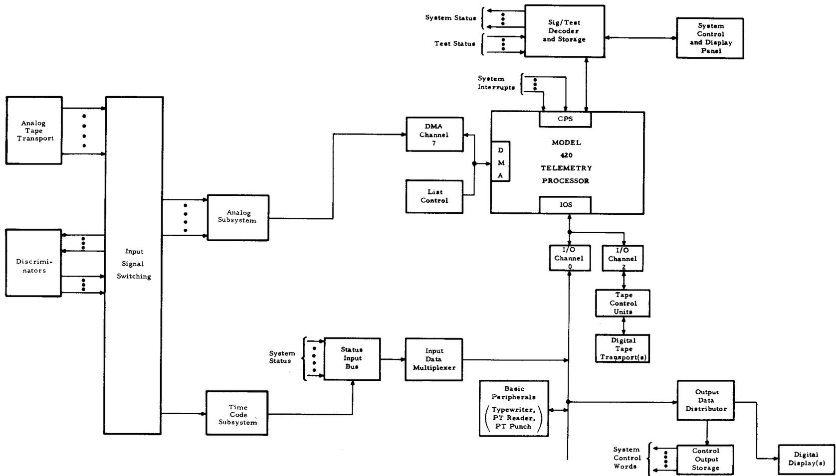
Figure 17. Model 8420 Configuration for Application Number Three (FM Conversion)
