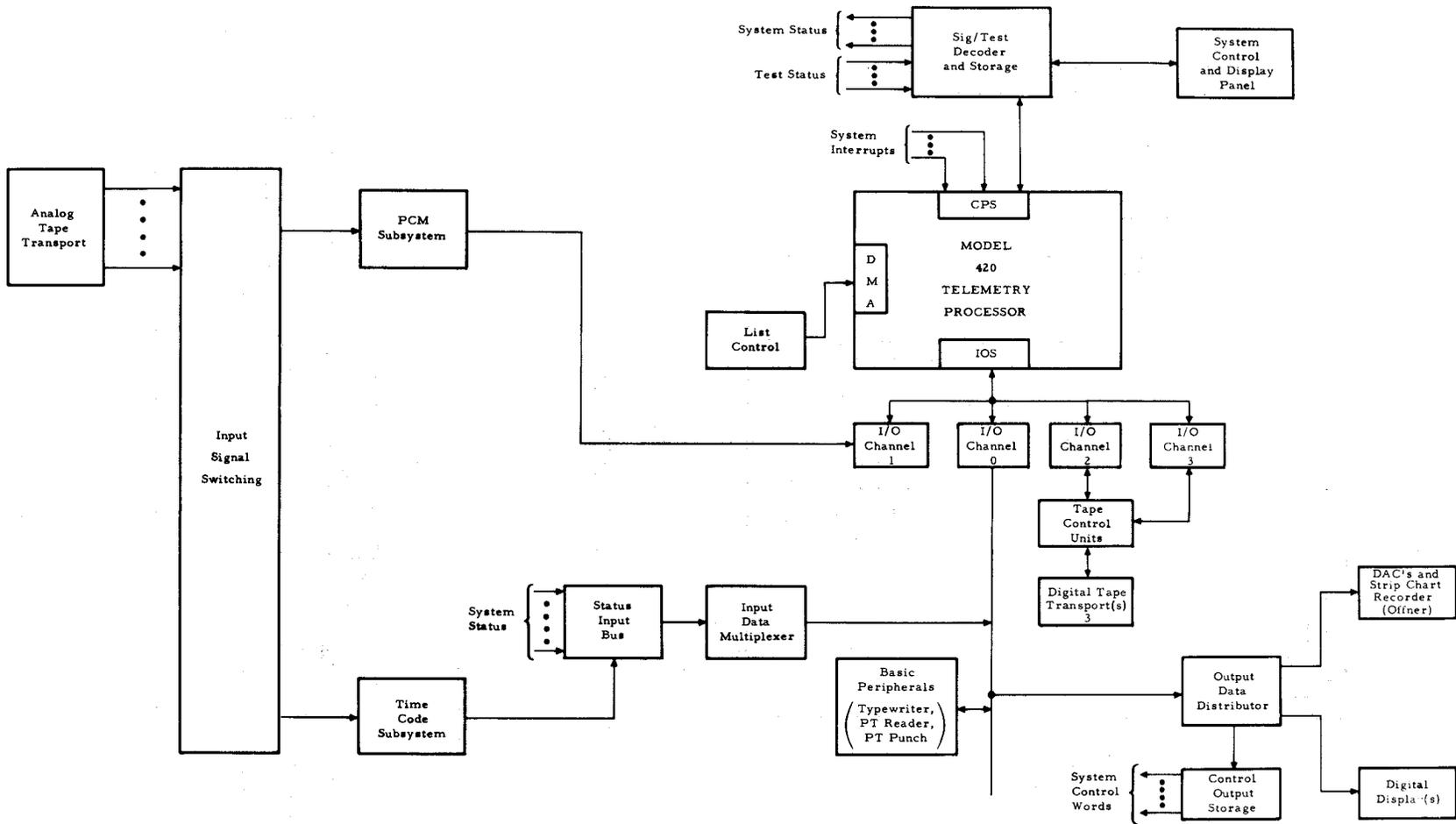
Figure 4. Model 8420 Configuration for Application Number One (On-Line Sort of PCM)
