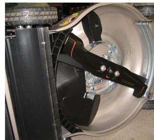
Figure 3. Rotary mower blade
