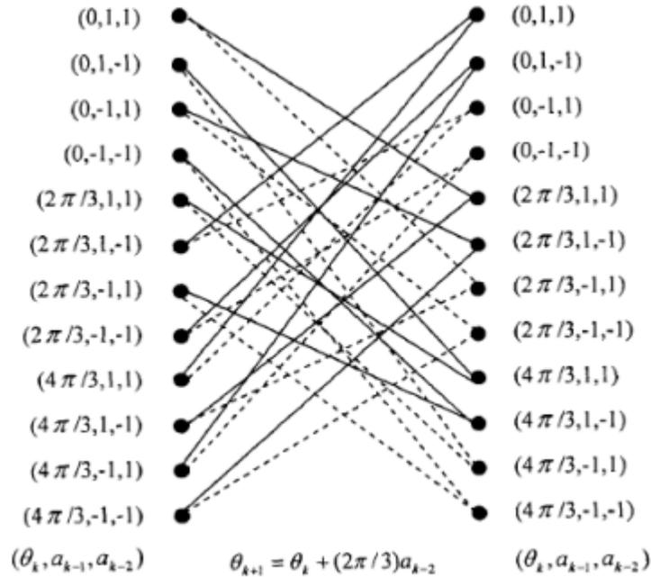
Figure 1. CPM trellis diagram ( $g(t) = 3RC$ ,  $h = 2/3$  and  $M = 2$ )
