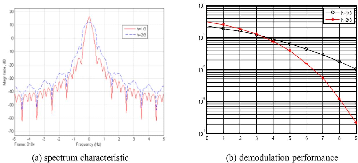
Figure 5. Performance with different modulation index  $h$
