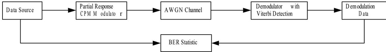
Figure 2. Block diagram of simulation
