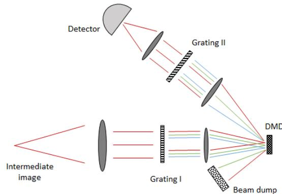
Figure 1: Schematic of the optical design for the AFSSI-C. Light from the scene enters the first arm of the system from the lower left, is dispersed and imaged onto the DMD, and then enters the second arm (where the dispersion is reversed) before detection.
