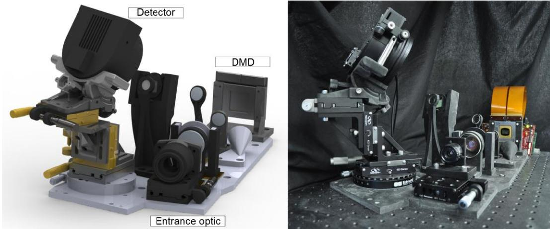
Figure 3: (Left): A rendering of the prototype design for the AFSSI-C; (Right): Prototype AFSSI-C with light restricting baffling removed.
