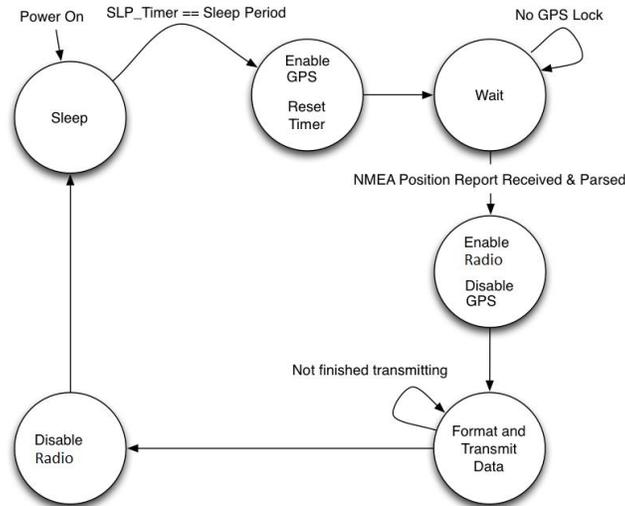
Figure 2: High Level Overview of System Operation
