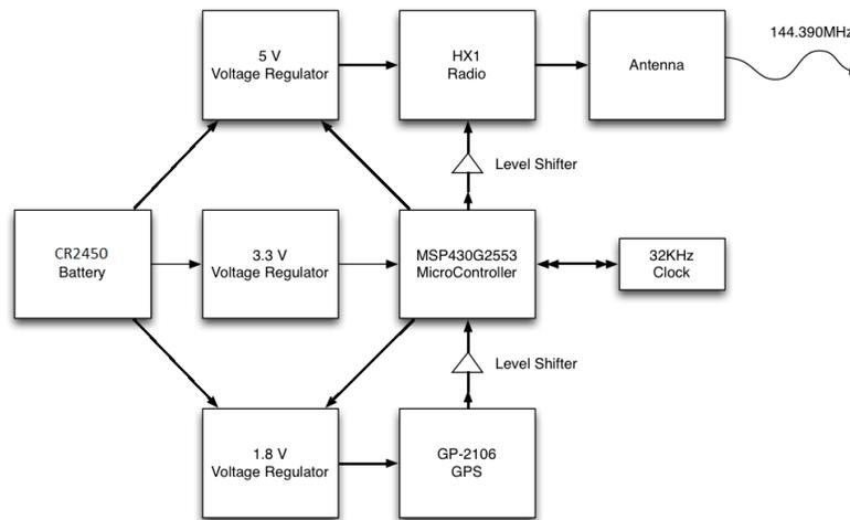
Figure 1: Transmitter Design Overview
