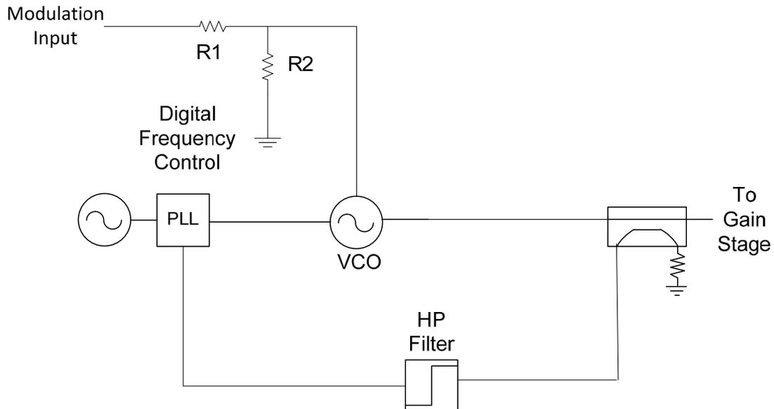
**Figure 1 – PLL/VCO Block Diagram**
