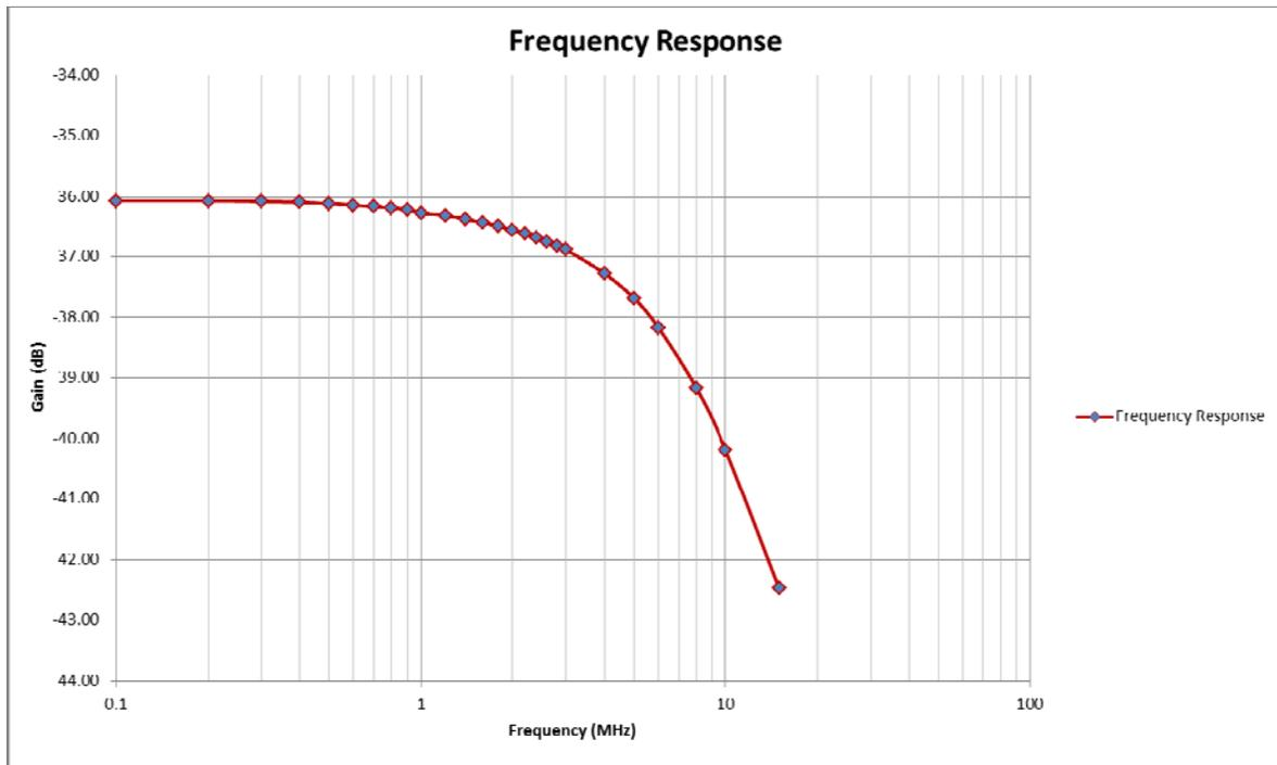
**Figure 6 – Frequency Response with R3=92 Ohms, R4=10K Ohms**
