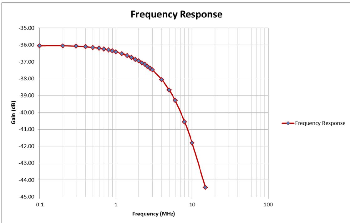
**Figure 5 – Frequency Response with R3 = 220 Ohms, and R4 Unpopulated**
