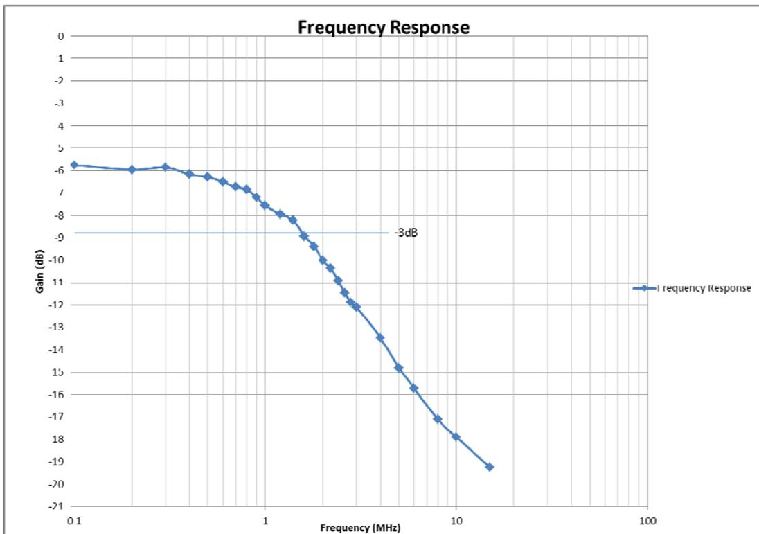
**Figure 7 – Measured Frequency Response of the Circuit in Figure 2**
