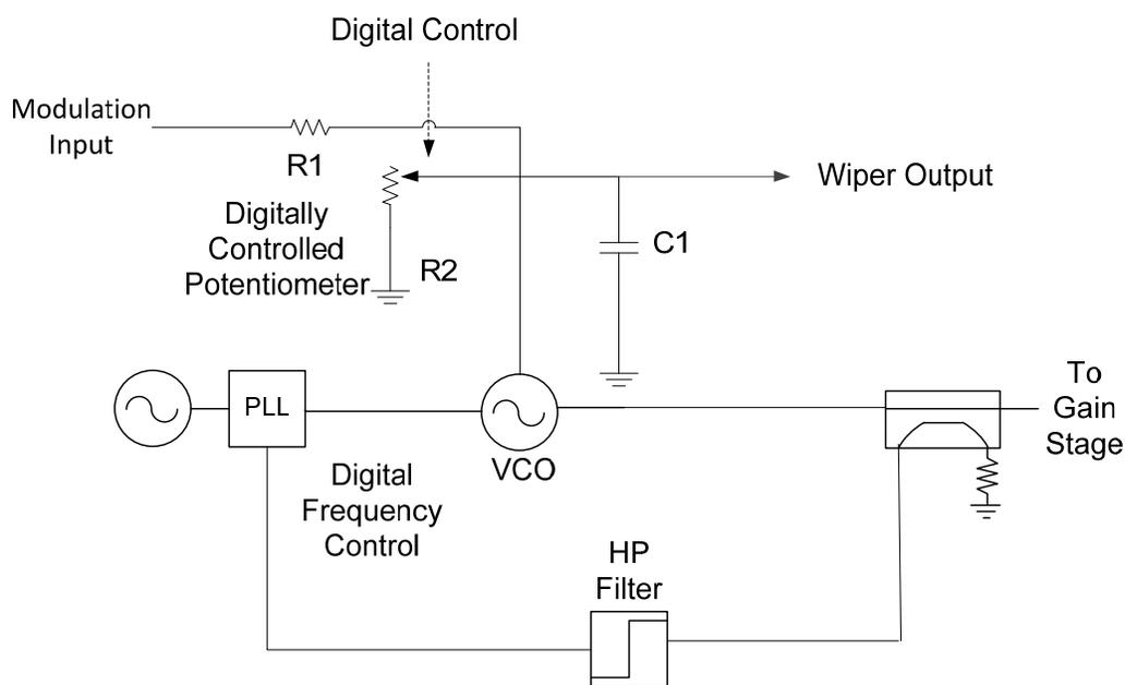
**Figure 2 – PLL/VCO Block Diagram with Digital Potentiometer**
