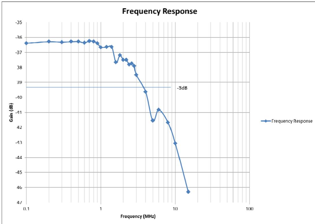
**Figure 8 – Measured Frequency Response of the Circuit in Figure 4, with  $R3 = 220$  Ohms,  $R4$  unpopulated**
