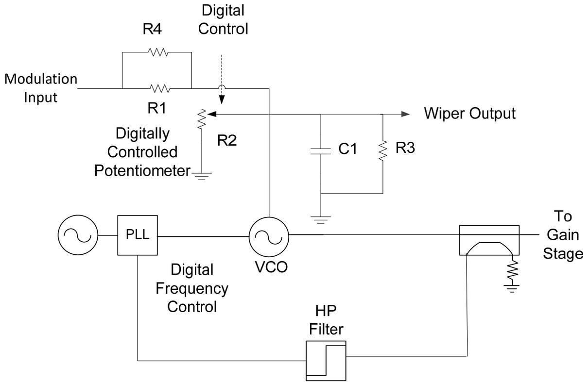
**Figure 4 – Potentiometer Circuit with Parallel Resistors**
