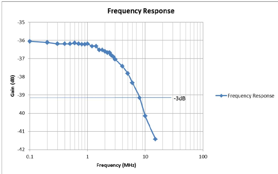
**Figure 9 – Measured Frequency Response of the Circuit in Figure 4, with R4 populated with 10K**
