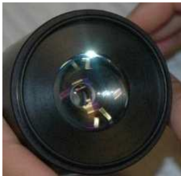
Figure 4.12: The eight element chromatic re-imaging optics (CRO) mounted in a lens barrel.
