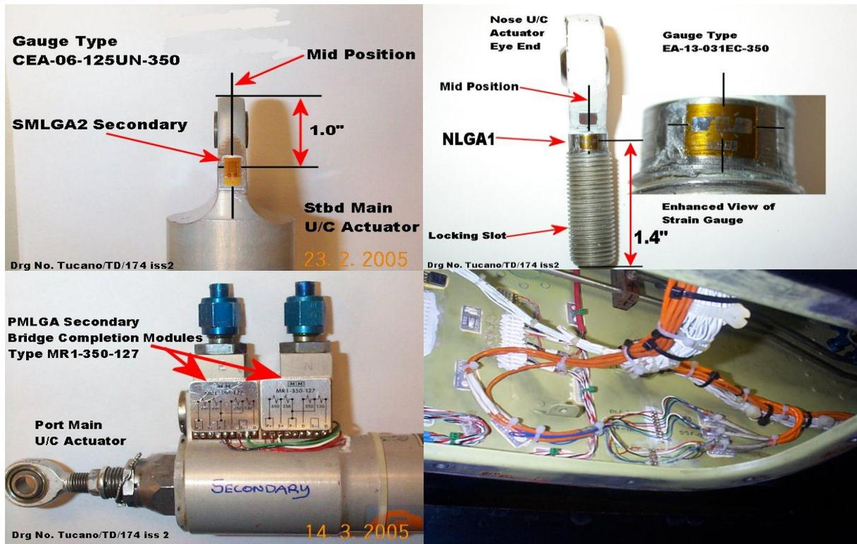
**Figure 1: Sensors and wiring considerations inform module selection**
