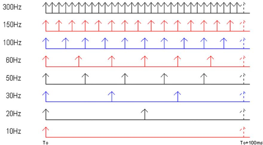
**Figure 2: Sampling different data rates in an acquisition cycle**
