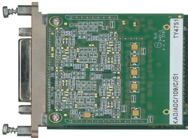
**Figure 3: Prototype uses an Acra KAM-500 form factor**
