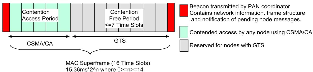
**Figure 2: Beacon-Enabled ZigBee Superframe**
