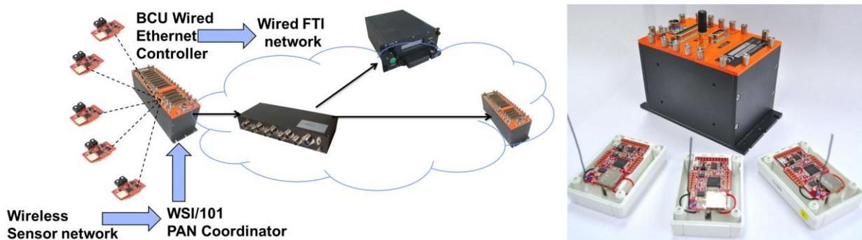
**Figure 3: WSN Configuration for Data Acquisition using WSI/101 PAN Coordinator User Module**
