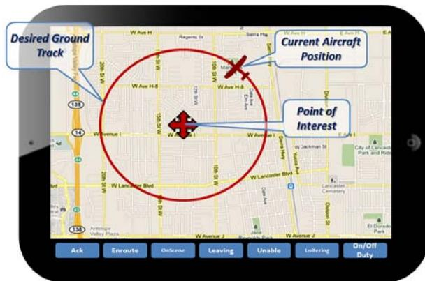
Figure 4 - Tasking the LEAPS Pilot
