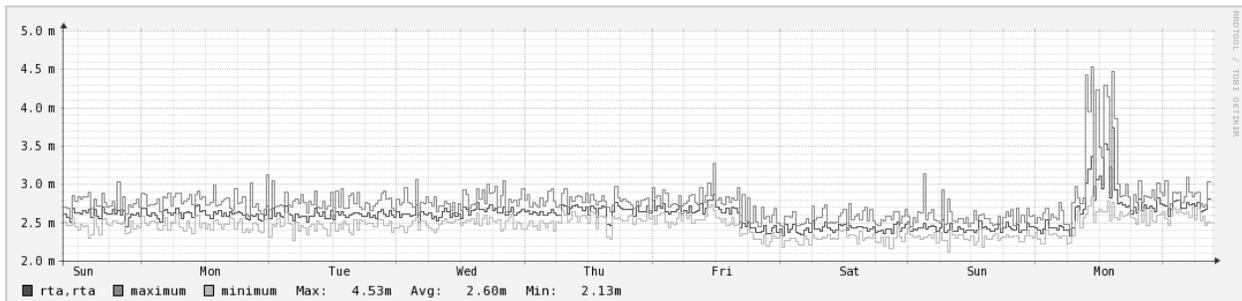
Figure 6 – Ping round trip time over the course of one week between the ATR Range Control Facility and the NASA Wallops Flight Facility site over a microwave network link showing high delay
