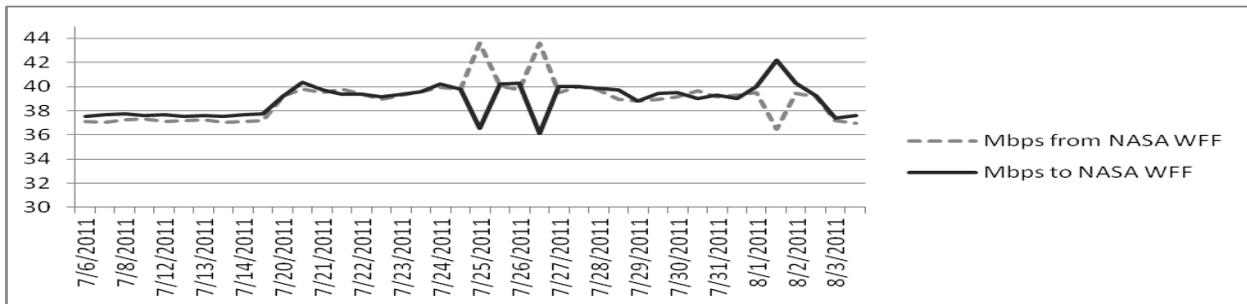
Figure 3 – Link throughput over the course of several weeks between the ATR Range Control Facility and the NASA Wallops Flight Facility over a microwave network link
