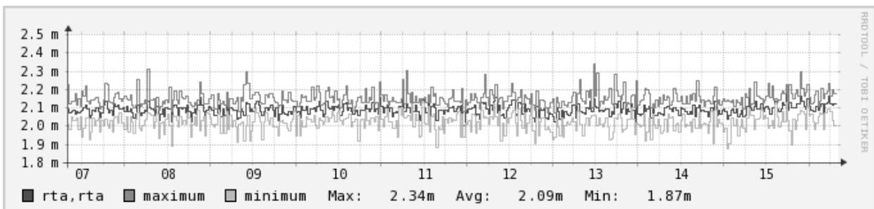
Figure 4 – Ping round trip time over the course of one week between the ATR Range Control Facility and the NASA Wallops Flight Facility site over a microwave network link
