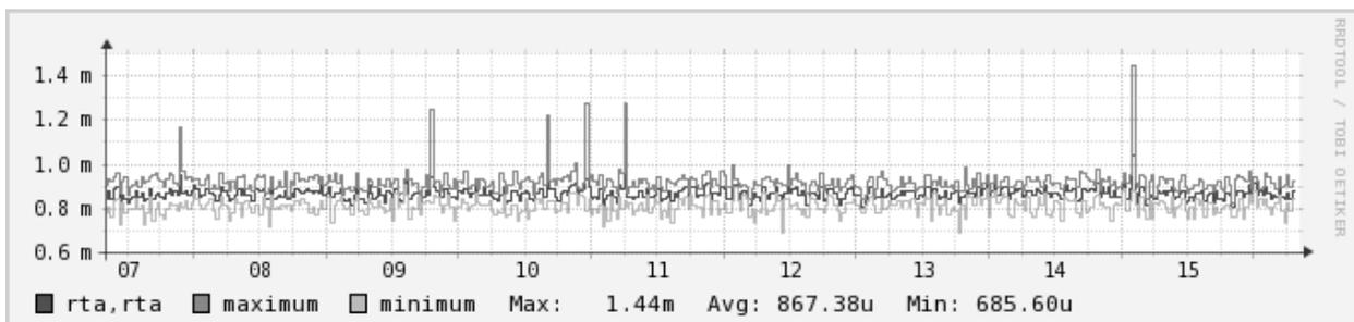
Figure 1 – Ping round trip time over the course of one week between the ATR Range Control Facility and a local antenna site over a fiber optic network link
