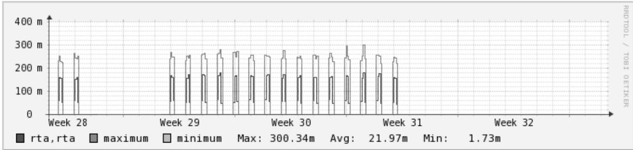
Figure 5 - Ping round trip time over the course of several weeks between the ATR Range Control Facility and the NASA Wallops Flight Facility site over a microwave network link
