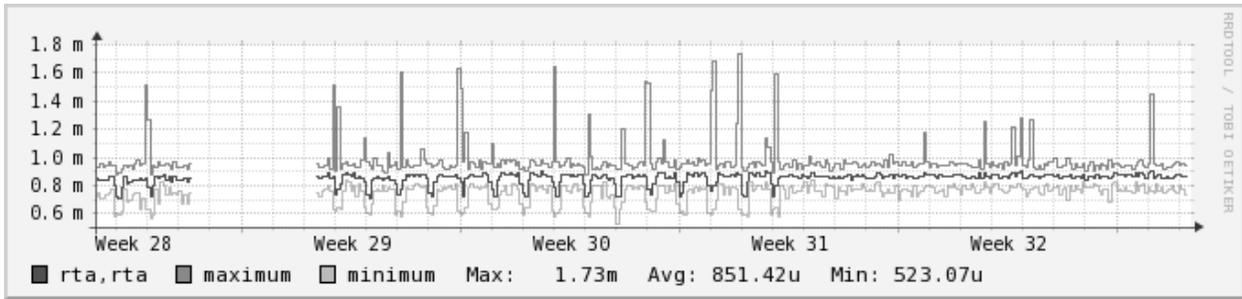
Figure 2 – Ping round trip time over the course of several weeks between the ATR Range Control Facility and a local antenna site over a fiber optic network link showing active testing
