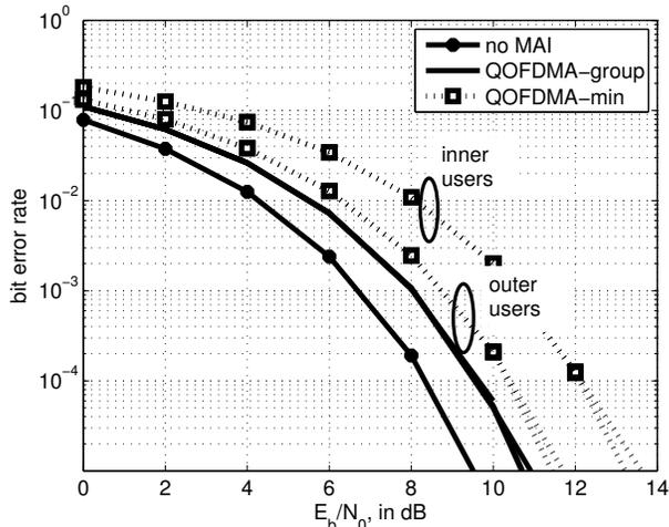
Figure 4: Performance comparison in the absence of frequency offsets due to oscillator and Doppler shifts in AWGN channel conditions.
