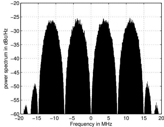
Figure 1: Power spectrum for FDMA at 5 Mbps bit rate. The occupied bandwidth 28.5 MHz.
