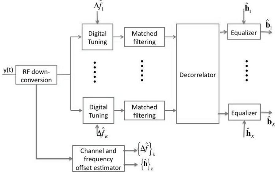
Figure 3: Receiver block diagram.
