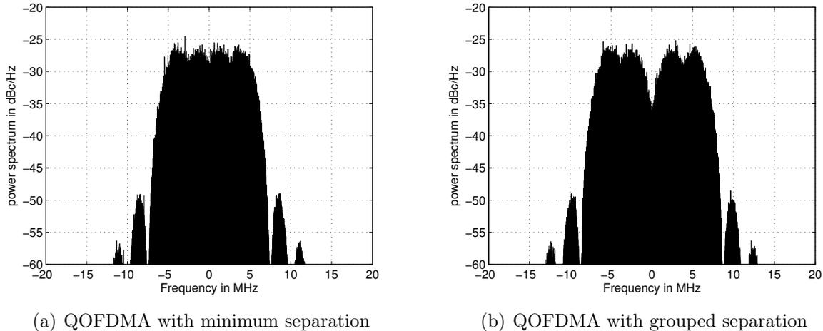
Figure 2: Power spectra for QOFDMA at 5 Mbps bit rate. The occupied bandwidth 13.5 MHz for QOFDMA with minimum separation, and 15 MHz for grouped separation.
