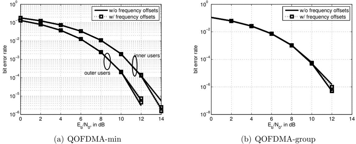
Figure 5: Average BER performance comparison averaged over frequency offsets due to oscillator and Doppler shifts in AWGN channel conditions.
