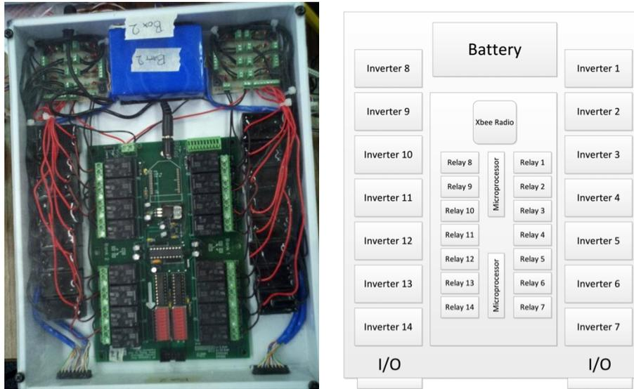
**Figure 2: An illustration of the controller box (left) and a block diagram showing the components (right).**
