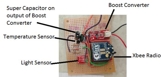
Figure 2: Picture of node showing major components and layout.
