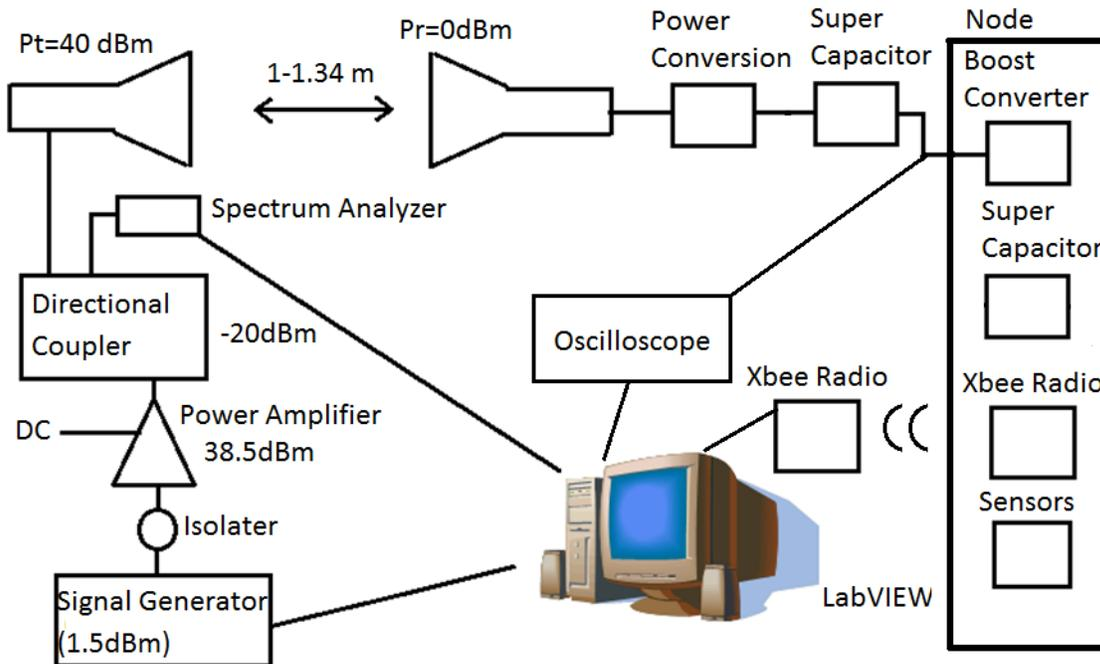
Figure 3: Test setup functional block diagram
