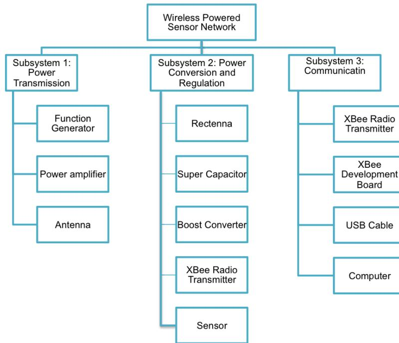
Figure 1: Functional decomposition of the system
