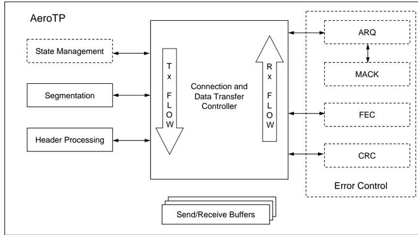
Figure 1: AeroTP implementation architecture
