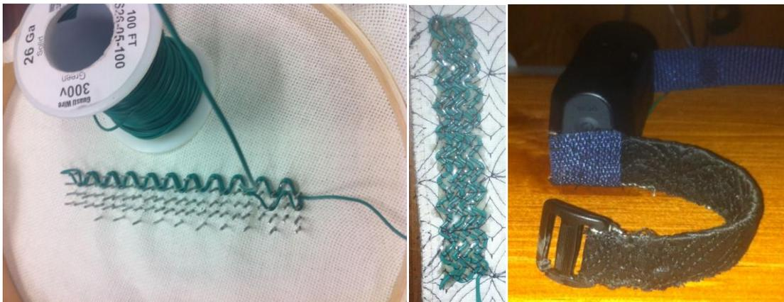
Figure. 5.1: Construction and Final Prototype Antenna (Black Collar)
