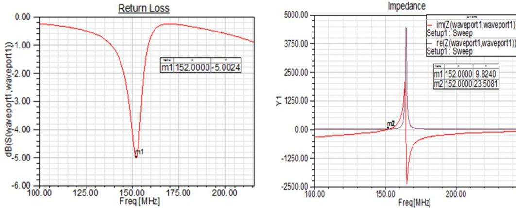
Figure. 4.2: The return loss and impedance of the final design
