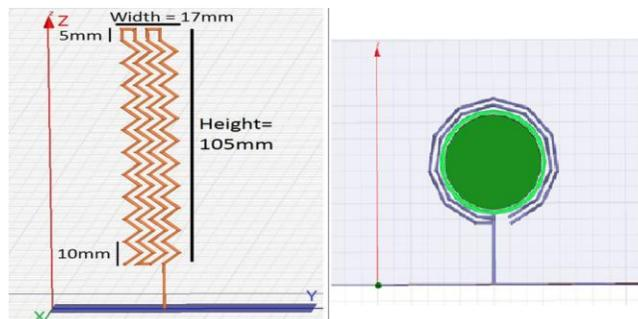
Figure. 4.1: Upright dimensions of the antenna, and side view of the curved antenna illustrating two layers
