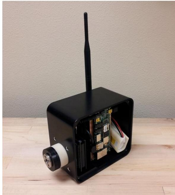
**Figure 7.** *Integrated RISA Camera with Anodized Enclosure.*
