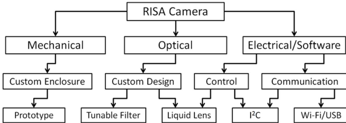
**Figure 1.** *RISA Camera High Level Design Subsystems.*
