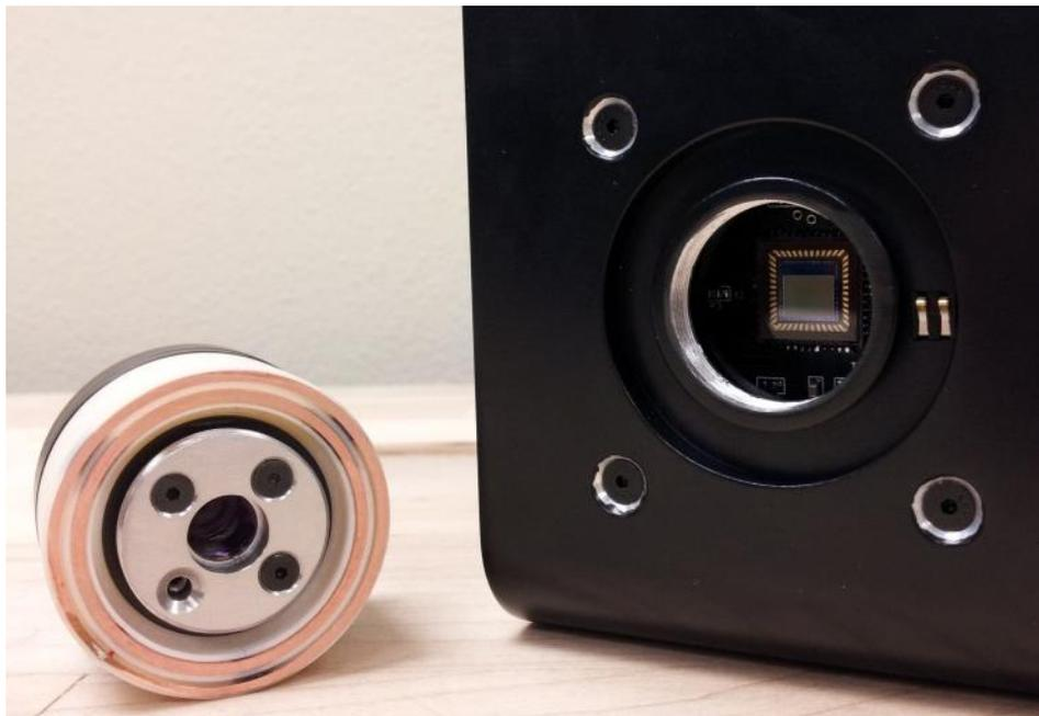
**Figure 5.** *Lens Barrel and Enclosure Showing Liquid Lens Electrical Contact Points.*
