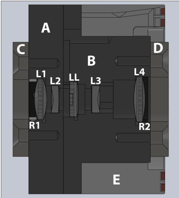
**Figure 6.** *Lens Barrel Annotated Design.*
