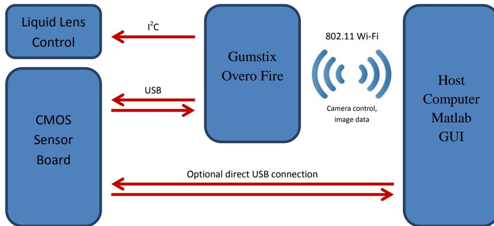
**Figure 3.** *Electrical System Block Diagram.*
