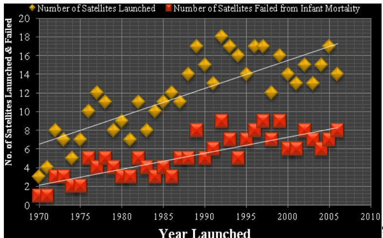
**FIGURE 3 THE PREMATURE FAILURE RATE OF MILITARY, COMMERCIAL AND NASA SATELLITES FROM 1970 THROUGH 2005 (FROST & SULLIVAN)<sup>5</sup>**
