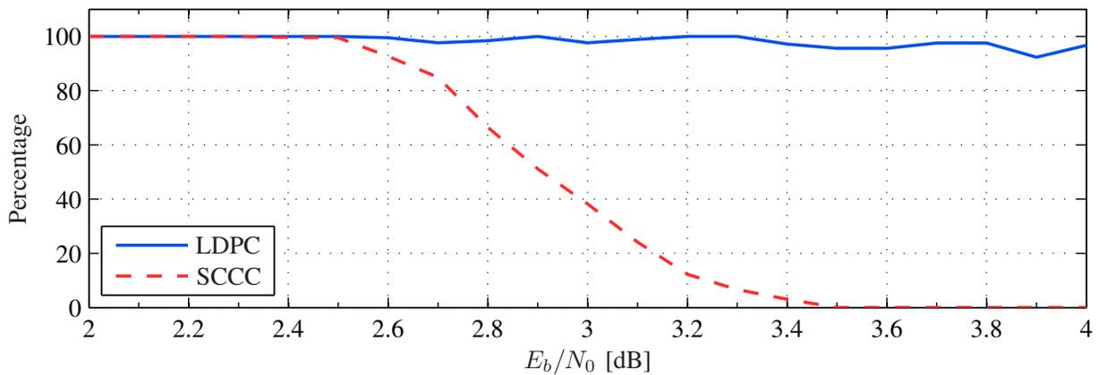
Figure 5: The percentage of phase slips that ultimately lead to decoded bit errors. In the case of LDPC, essentially all phase slips result in decoded bit errors. In the case of SCCC, as  $E_b/N_0$  increases, the SCCC decoder is better able to correct the phase slip errors and at some point the phase slips no longer contribute to the BER.
