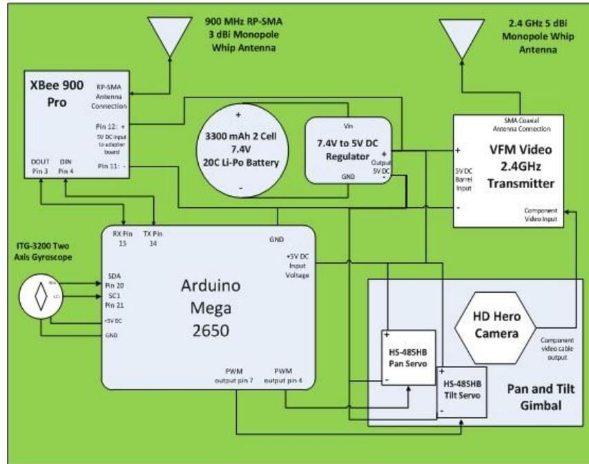
Figure 2: Level 2 block diagram of on board system.
