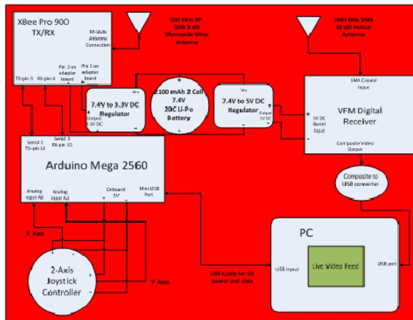
Figure 4: Level 2 block diagram of ground station subsystem.
