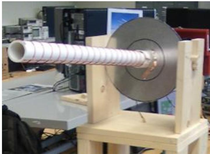
Figure 3: 18 dBi helical receiver antenna.
