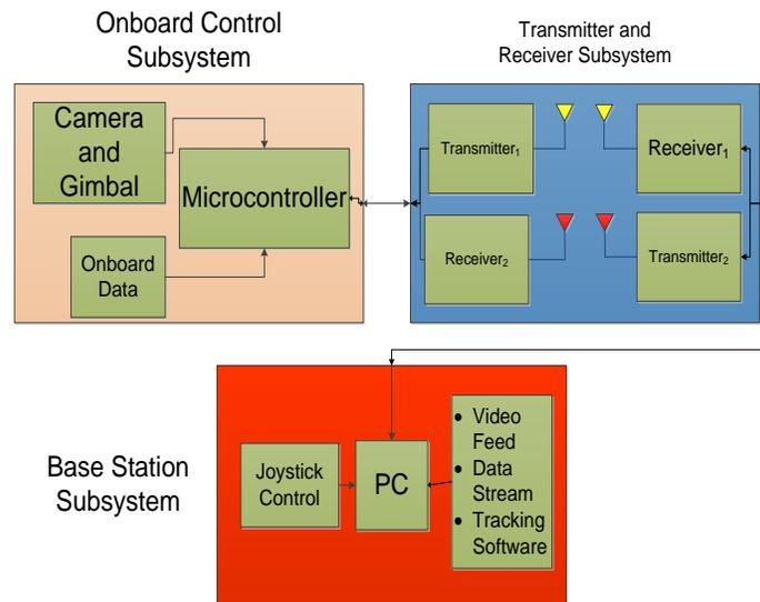
**Figure 1: Block diagram of three sub-systems.**
