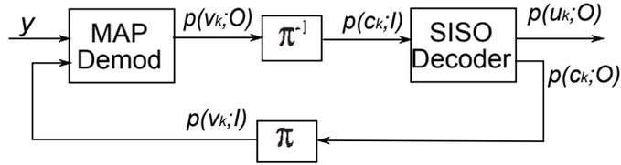
Fig. 2. Block diagram of receiver.
