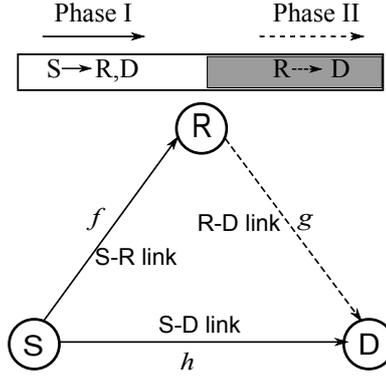
Fig. 1. Cooperative Communication model with a source, destination and a single relay.
