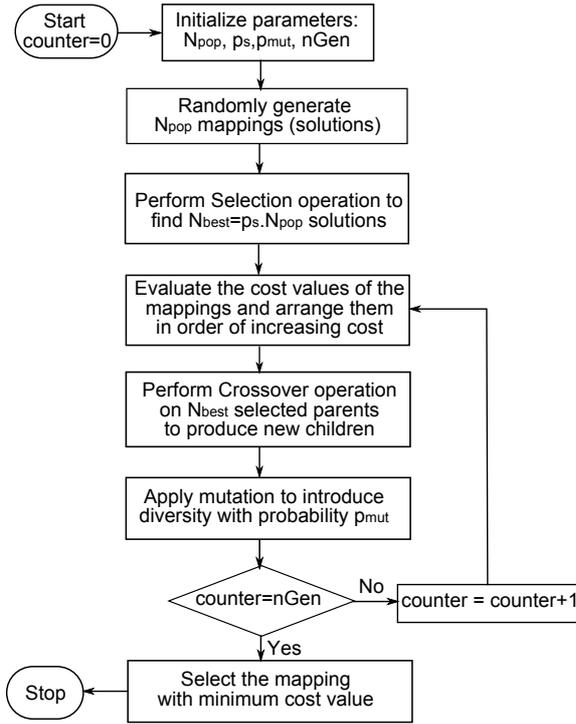
Fig. 3. Flow chart for the GA to find the optimized symbol mapping.
