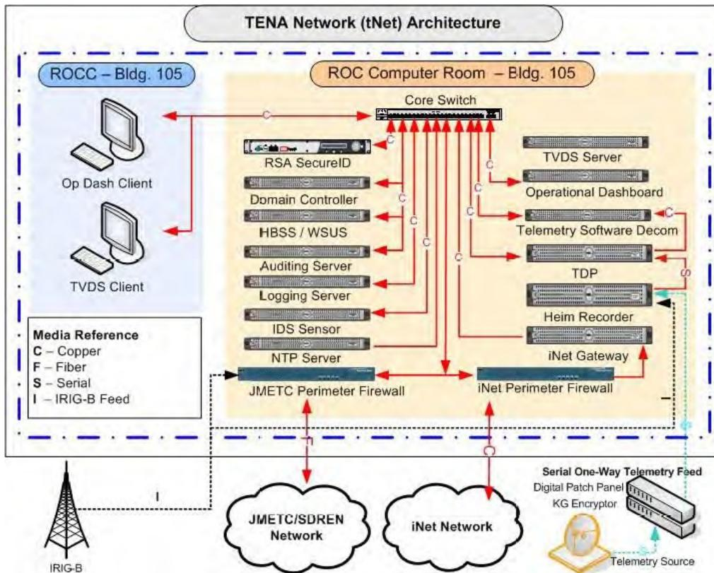
(Figure 2. Test Bed Architecture)
