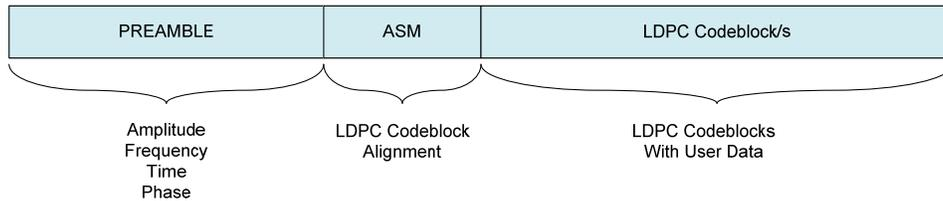
Figure 5. Burst Transmission Structure from RANS
