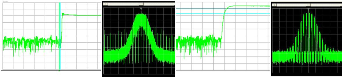
Figure 4. Example of fast rise time with spectral splatter (left) and controlled rise time with no spectral splatter (right).
