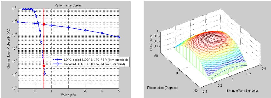
Figure 7. Uncoded  $P_c$  and Coded CBER (left), Sync error surface (right)
