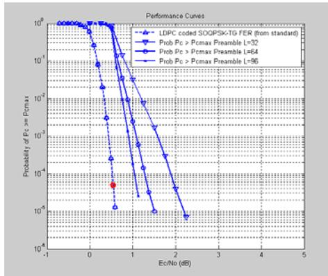
Figure 8. Probability that  $P_c > P_{c,max}$  versus  $E_c/N_0$  for various preamble lengths
