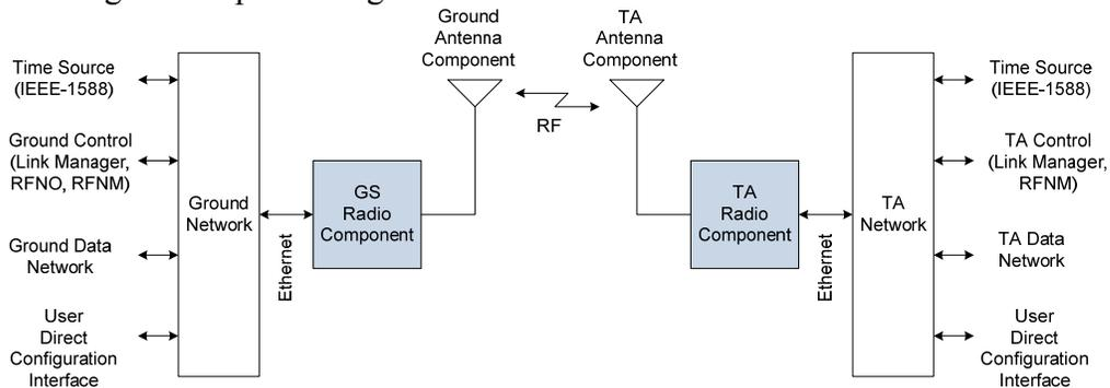
Figure 2. Simplified Block Diagram of RANS Radio Components
