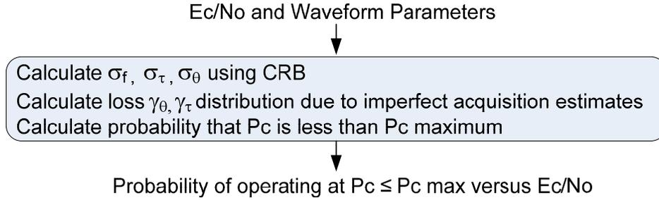
Figure 6. Calculation procedure for determining the performance margin versus SNR
