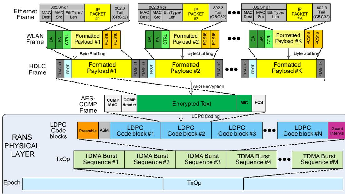
Figure 3. Message processing flow in RANS
