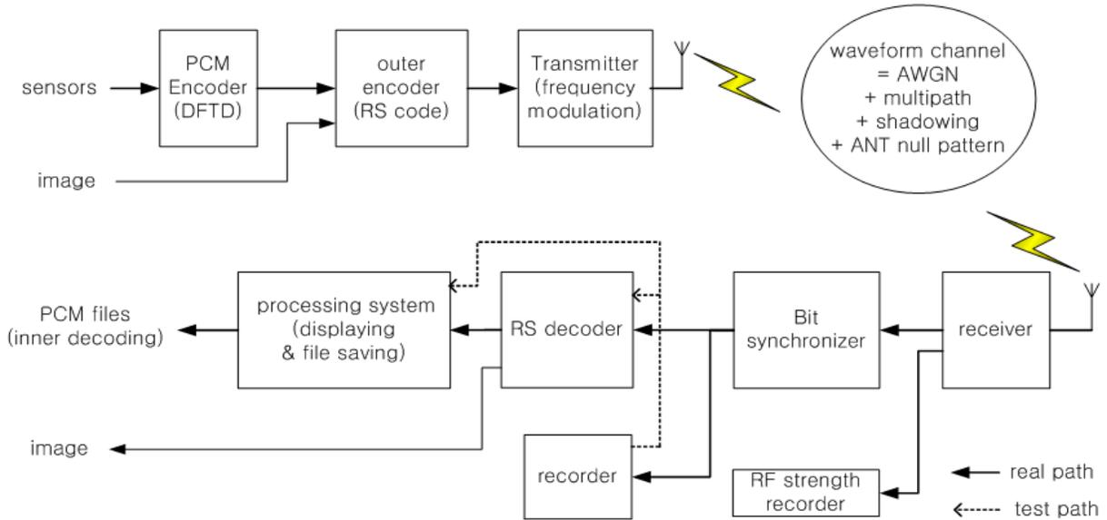
Figure 1: Block diagram of the overall scheme.
