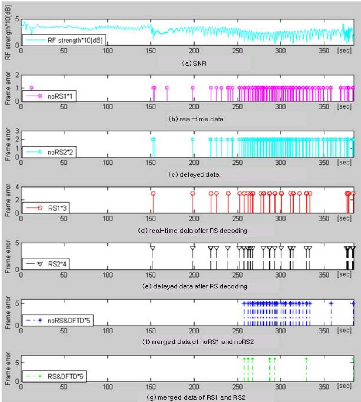
Figure 6: A comparison of the numbers of error frames.
