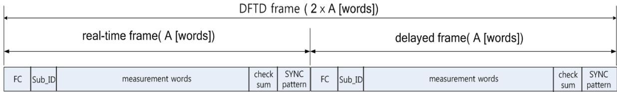
Figure 3: DFTD frame structure.
