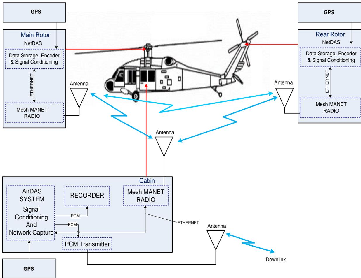
**Figure 3: Wireless Rotor Data Acquisition System (PCM with Ethernet Capture Solution)**
