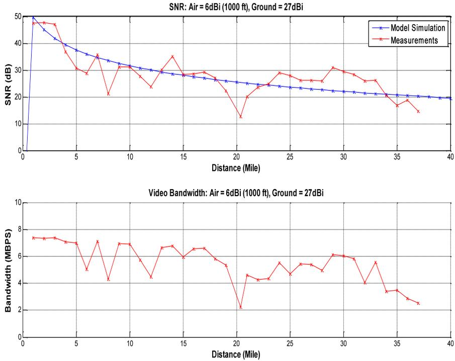
**Figure 5: SNR and Video Bandwidth vs. Distance for the Test Case #1 at 1,000ft Altitude**
