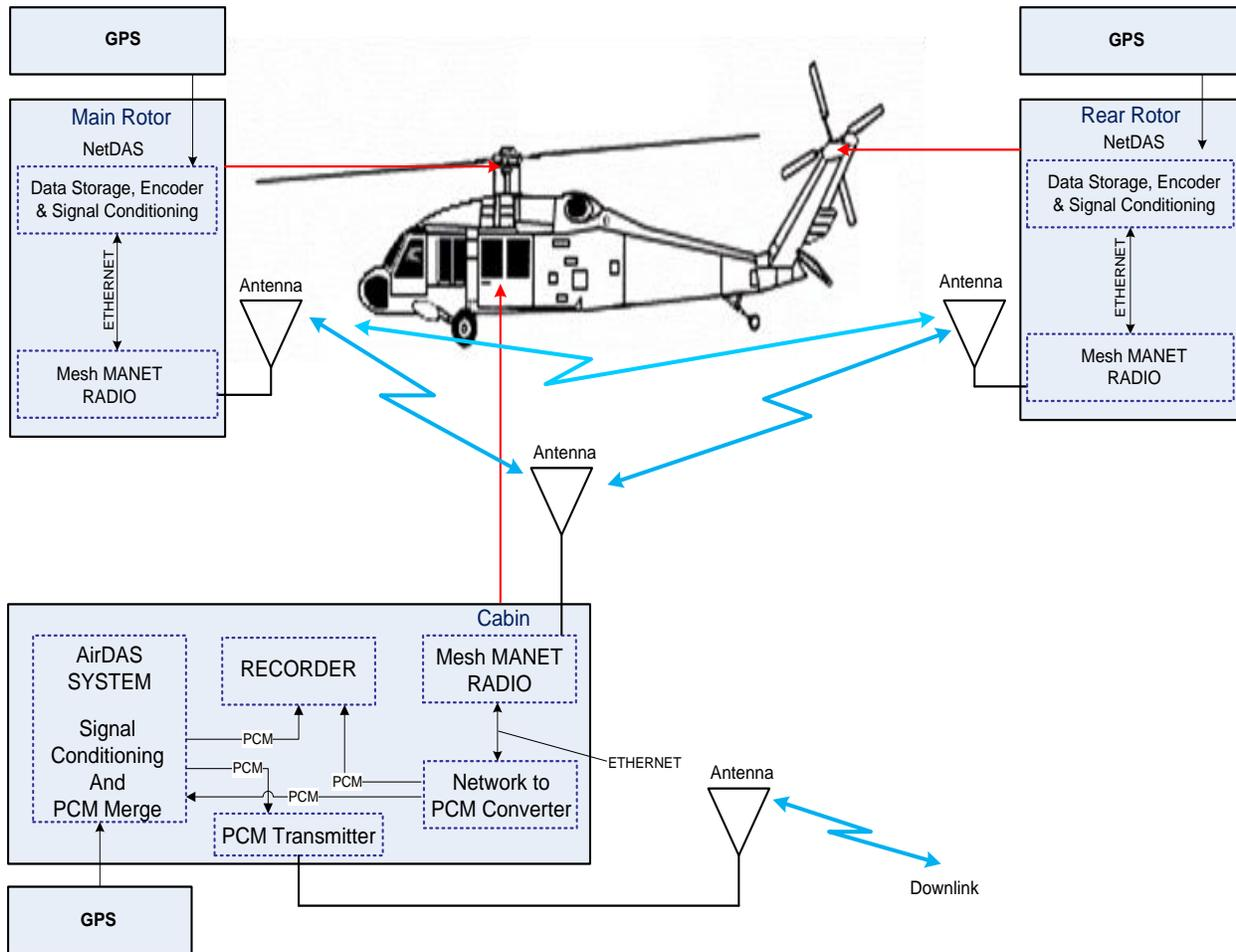
**Figure 2: Wireless Rotor Data Acquisition System (PCM with Merge Solution)**
