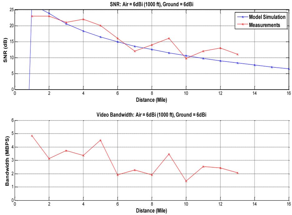
**Figure 6: SNR and Video Bandwidth vs. Distance for the Test Case #2 at 1000ft Altitude**
