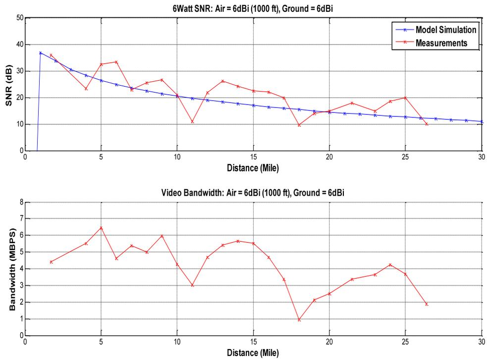
**Figure 7: SNR and Video Bandwidth vs. Distance for the Test Case #2 with an additional 6W Power Amplifier at the Helicopter Radio at 1000ft Altitude**
