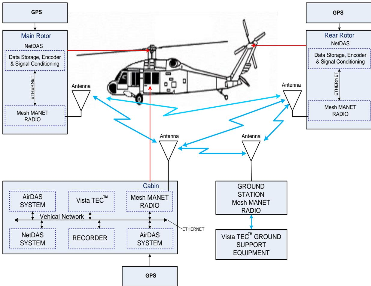
**Figure 1: Wireless Rotor Data Acquisition System (Network Solution)**
