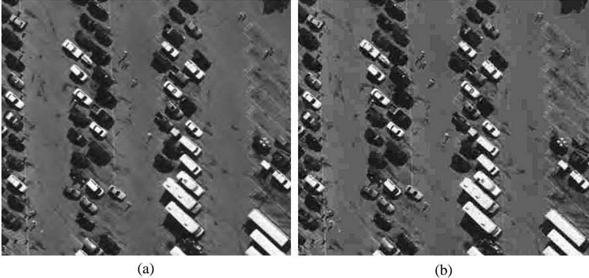
**Figure 1.** Images encoded with (a) JPEG2000 and (b) JPEG at the same bitrate (0.350 bits-per-pixel (bbp)). The JPEG image has the perceptually more distracting blocking artifacts.
