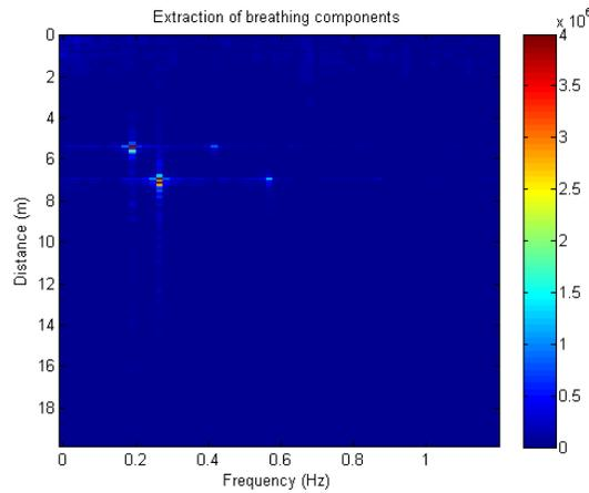
Figure (3): 2D spectrum of the data sequences from one transceiver pair
