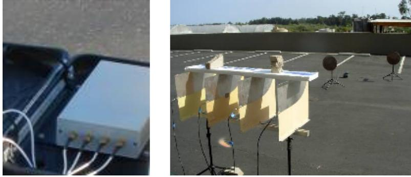
Figure (1): 4-antenna radar unit and the setup of the field experiment
