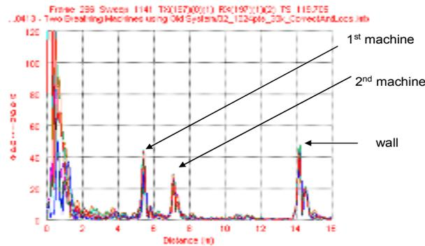
Figure (2): A range profile from one transceiver pair
