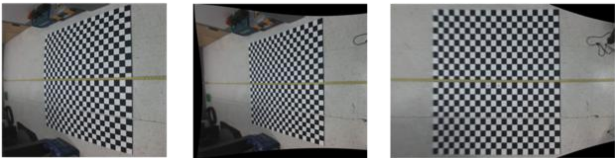
Figure 12: Original Image, Corrected Barrel Distortion, and Corrected Keystone Distortion.
