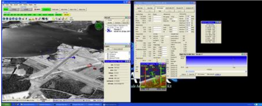
Figure 10: The Piccolo Command Center (PCC) Graphical User Interface
