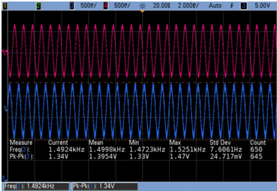
Figure 7- Input and output of the filter implemented on Xilinx Spartan-3 FPGA. Cutoff frequency 3 kHz. Sine wave 1.5 kHz
